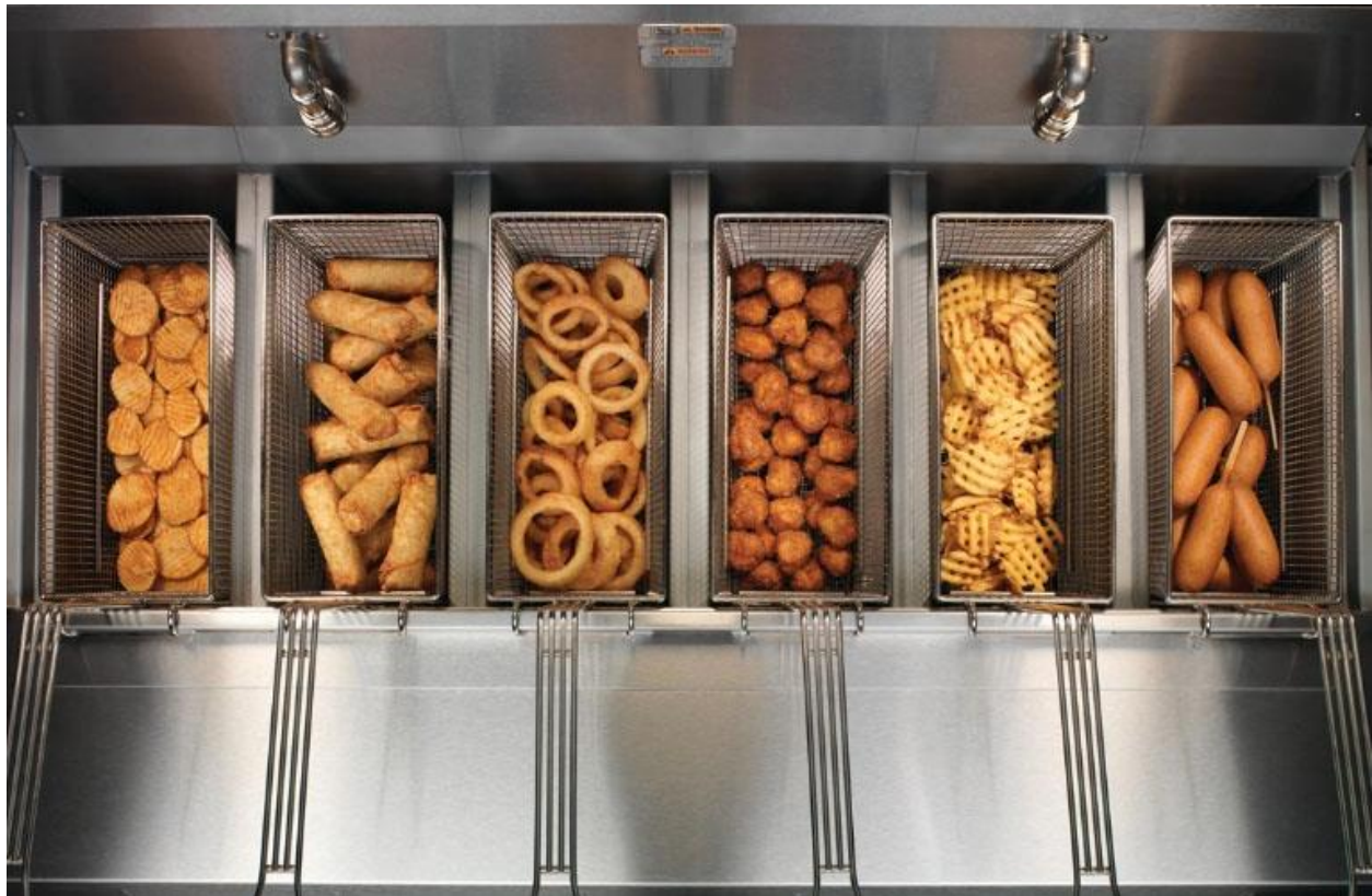
Figure 1 Commercial Six Bank Multi-Vat Fryer
