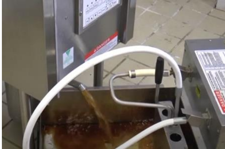
Figure 2 Fryer Oil Drained into the Filtration Tank Before Being Pumped Through a Filter
