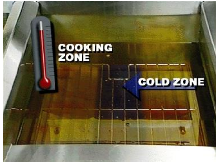
Figure 11 Demonstration of a Commercial Fryer Cold Zone with Oil Filled
