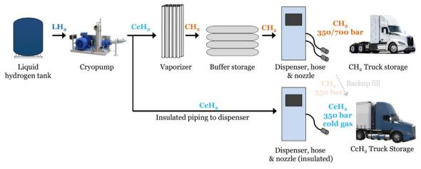
This highlights one of the greatest advantages to  $CcH_2$  over  $LH_2$ :  $CcH_2$  can use the same cryopump as H35 and H70. This is very different from trucks with onboard  $LH_2$  storage, which require a distinct, separate fueling pump.
