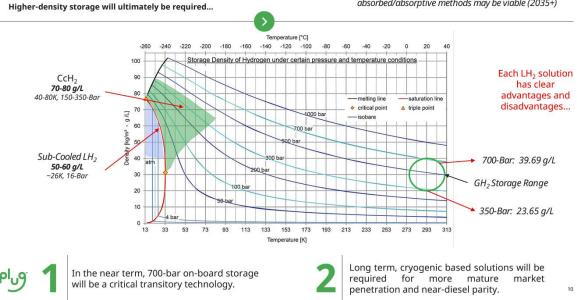
It is important for hydrogen refueling stations to consider future onboard hydrogen storage technologies such as CcH<sub>2</sub>. **Hydrogen refueling stations should be future-proofed**, built to enable fueling of multiple hydrogen storage technologies: they should have the ability to conduct 700 bar refueling today and be setup to easily accommodate refueling of other, emerging hydrogen storage methods in the future (such as CcH<sub>2</sub>).
