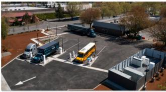
Left: Example of MHD vehicle attempting to utilize existing EV infrastructure catering only to light-duty passenger vehicles. Right: Successful implementation of dual purpose pull-though charging infrastructure able to accommodate all vehicle classes at Portland's Electric Island.
