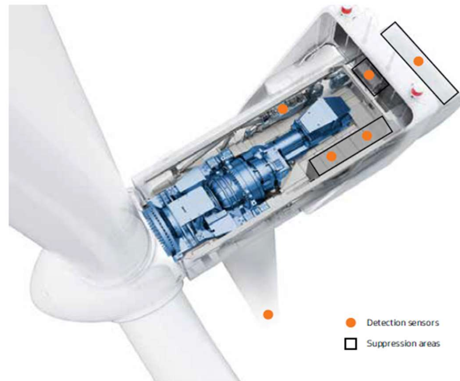
Illustration of fire detection and suppression system placement in a V136-3.45 MW *
