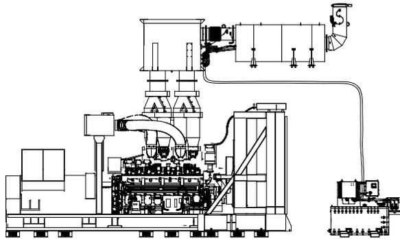
KDxxxx- 4 designates a 60 Hz generator set with a Tier 4 EPA-Certified engine.
