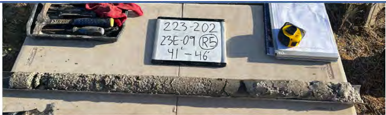
23E-09 Run 5 From 41.0 feet to 46.0 feet
