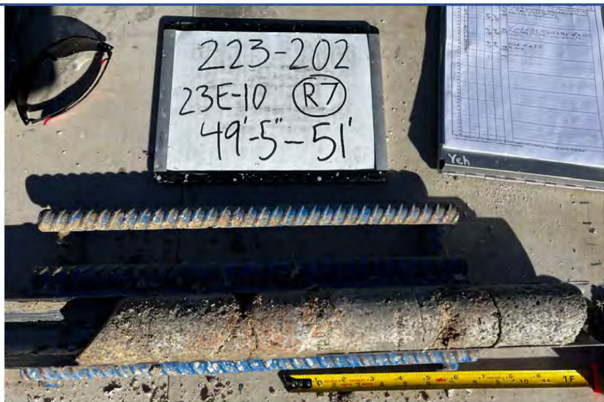
23E-10 Run 7 From 49.5 feet to 51.0 feet
