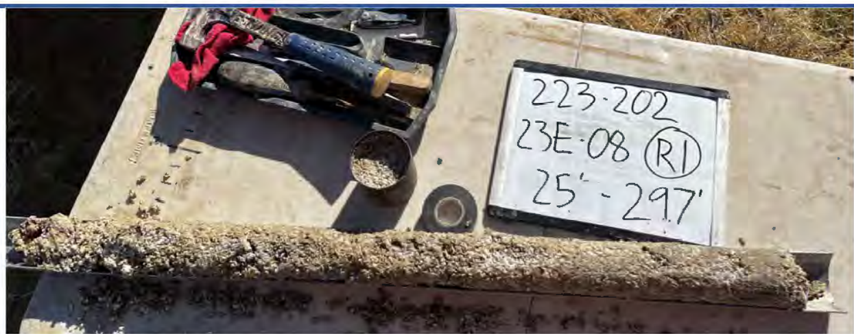
23E-08 Run 1 from 25.0 feet to 29.7 feet
