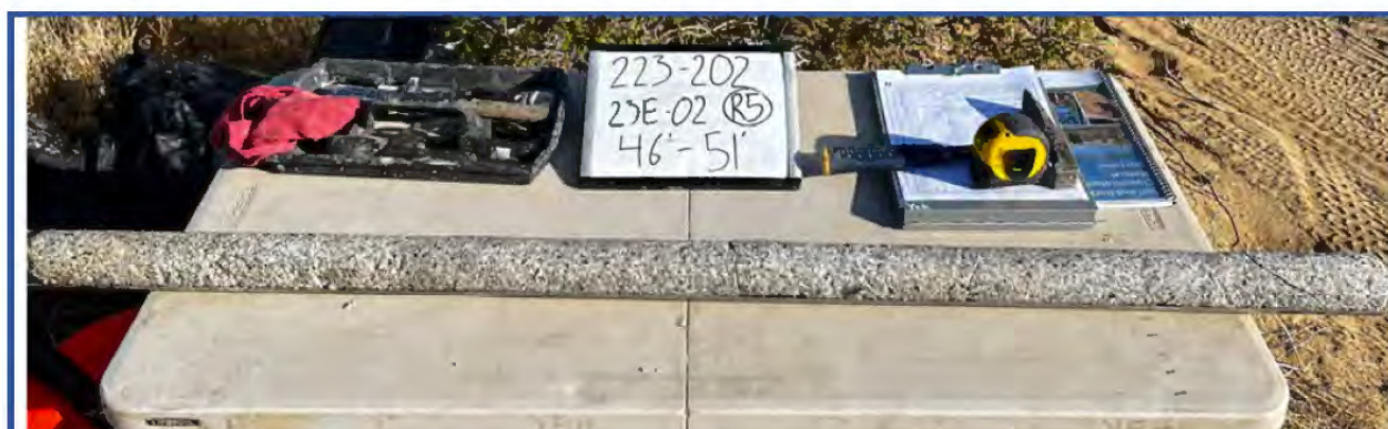
23E-02 Run 5 from 46 feet to 51 feet
