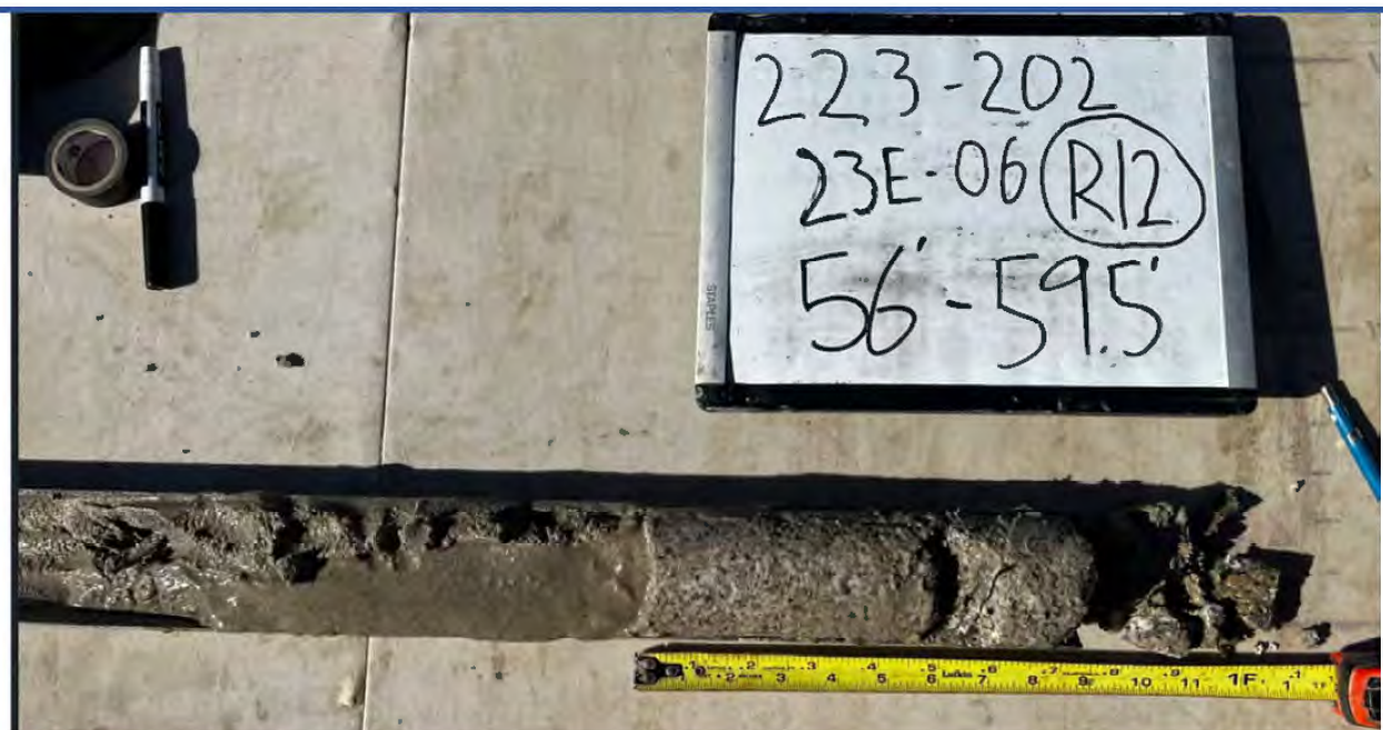
23E-06 Run 12 From 56.0 feet to 59.5 feet
