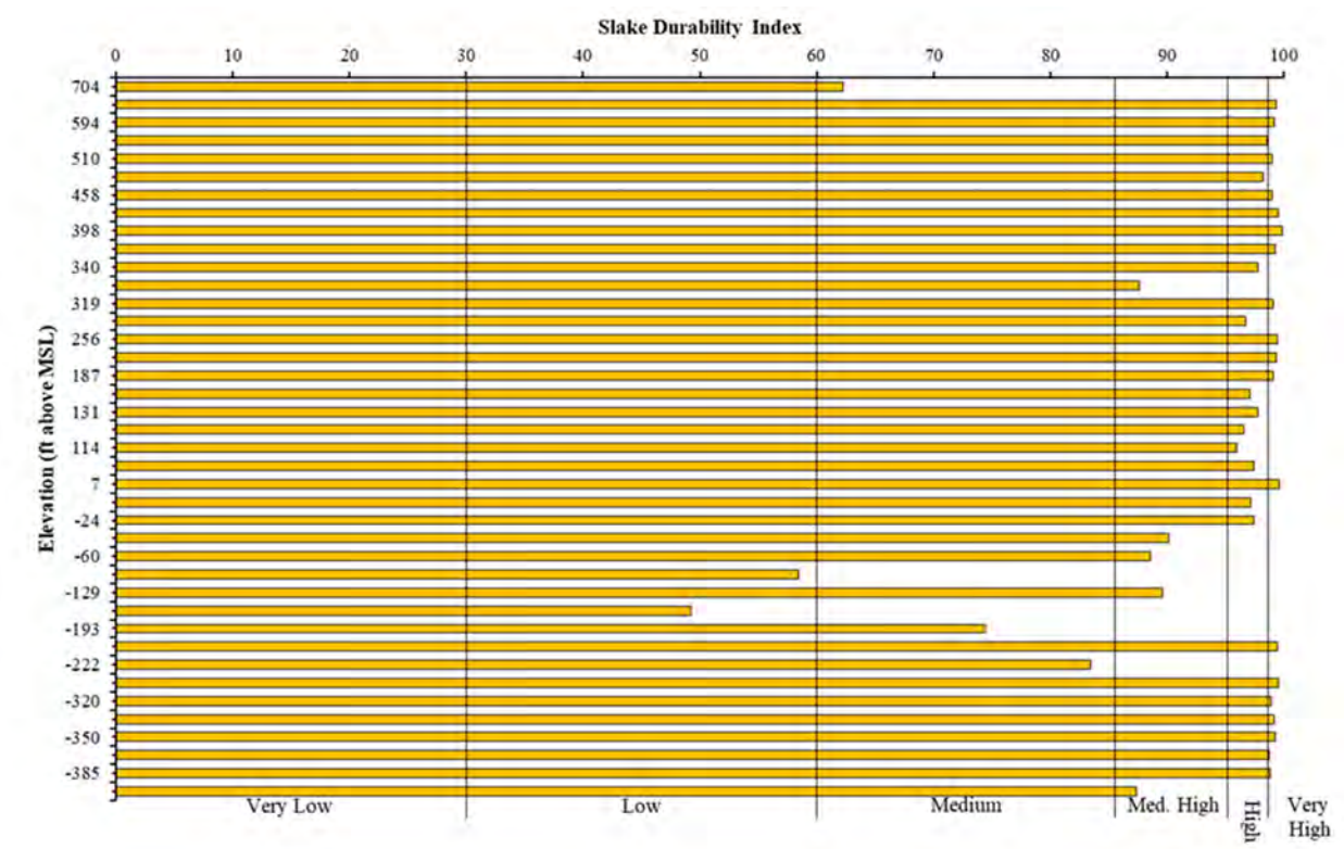
Figure 4-5. Slake Durability Index Recorded in Core Hole ZEV-CH-02-23
