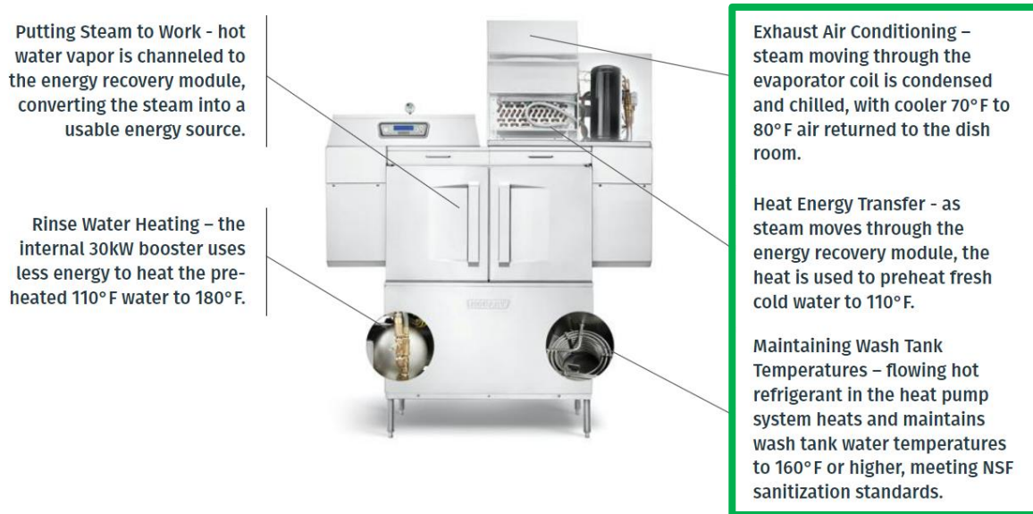
Figure 16: Heat Pump Exhaust Heat Recovery Machine Diagram
