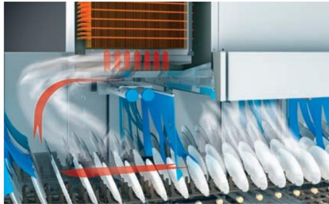
Figure 15: Flight-type machine heat recovery system at the exit of the machine.
