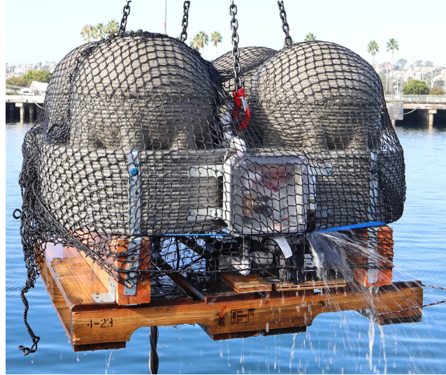
Fig. 3: RCAM tested a 3D printed and test its multi-sphere MPH in the Port of Los Angeles.
