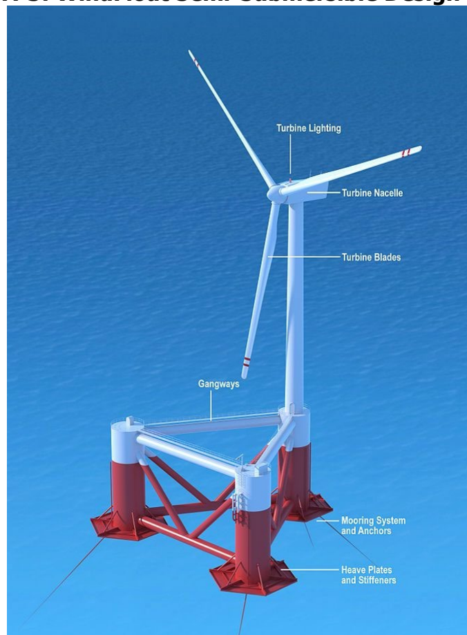
Figure A-3: WindFloat Semi-Submersible Design Concept
