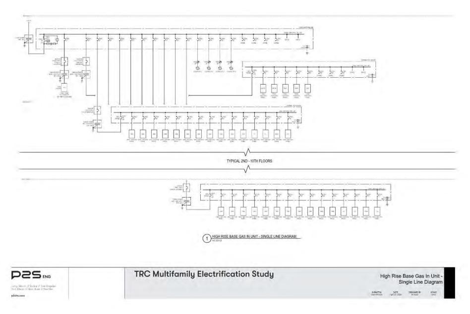
Figure 57: High-rise mixed use base case electrical SLD.
