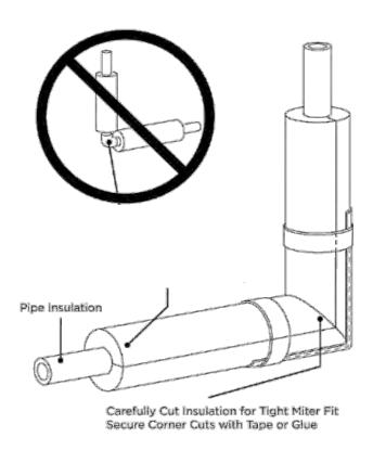
Figure 3: Illustration of improper and proper elbow insulation.
