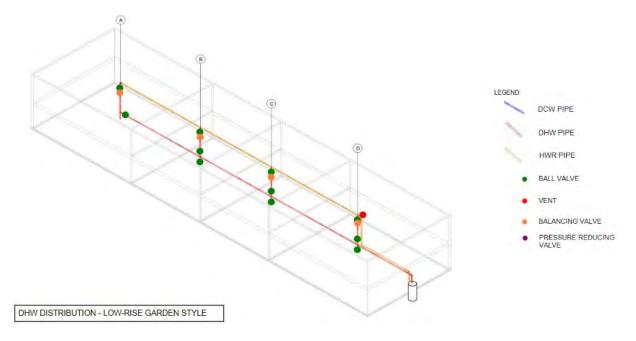
Figure 26: Low-rise garden style domestic hot water piping schematic with appurtenance locations.
