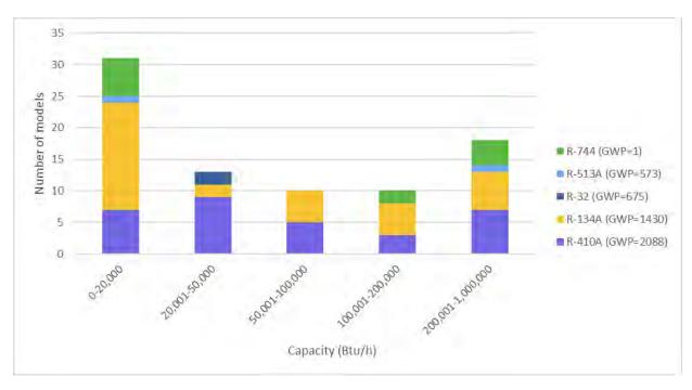
Figure 15: Air source HPWHs: refrigerant per system capacity.
