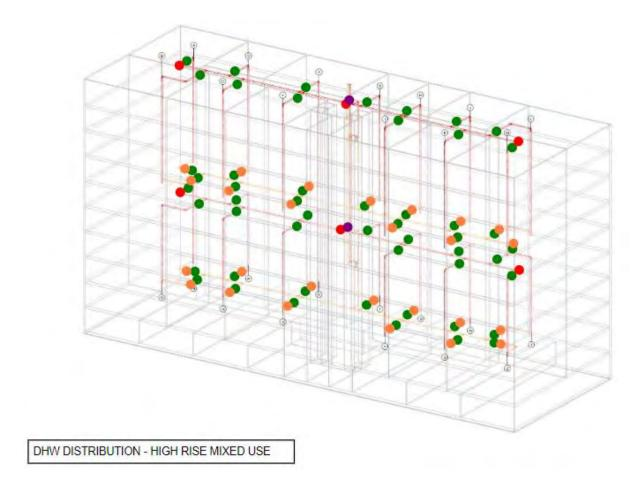
Figure 34: High-rise domestic hot water piping schematic with appurtenance locations.
