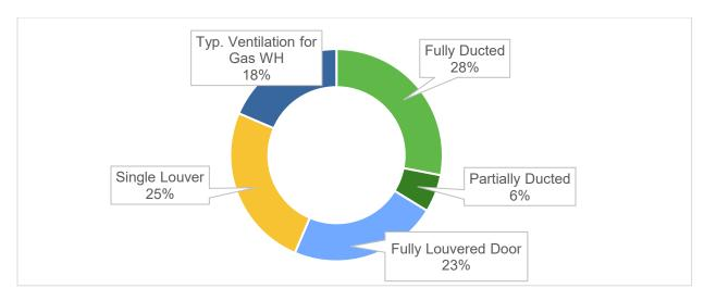
Figure 20: HPWH ventilation methods used in reviewed designs.
