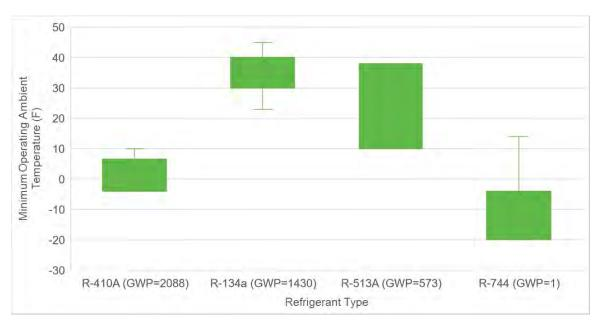
Figure 5: Refrigerant vs. minimal HPWH operating ambient air temperature.
