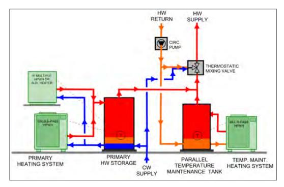
Figure 10: Single-pass primary with multi-pass in parallel for temperature maintenance system (Ref: NEEA, 2022).
