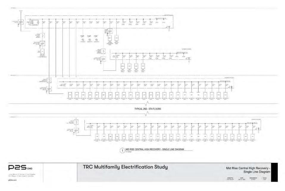
Figure 56: Mid-rise mixed use central high-recovery HPWH electrical SLD.
