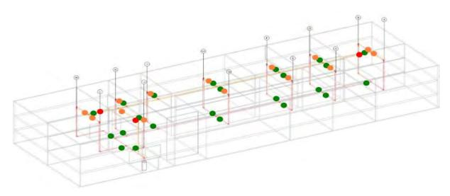
Figure 27: Low-rise loaded corridor domestic hot water piping schematic with appurtenance locations.
