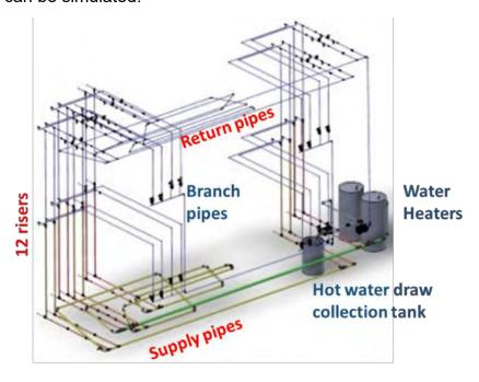
Figure 60: Folded design of test recirculation system.
