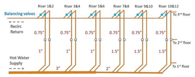
Figure 59: Schematics of recirculation distribution system for testing.
