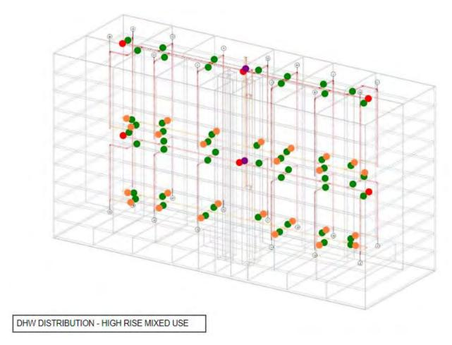
Figure 29: High-rise domestic hot water piping schematic with appurtenance locations.
