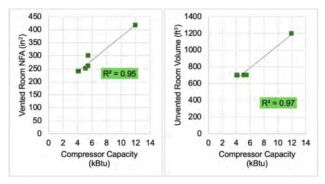
Figure 41. Manufacturer ventilation requirements by compressor capacity.
