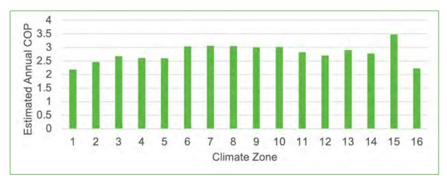
Figure 42. Estimated annual COP for HPWHs in small exterior closets with ventilation grilles based on laboratory test results.
