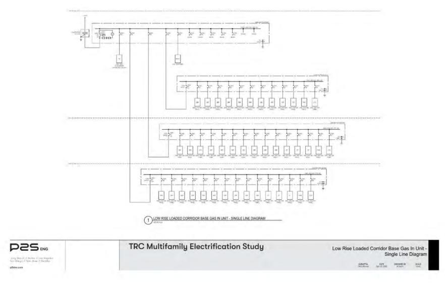
Figure 53: Low rise loaded corridor base case electrical SLD.
