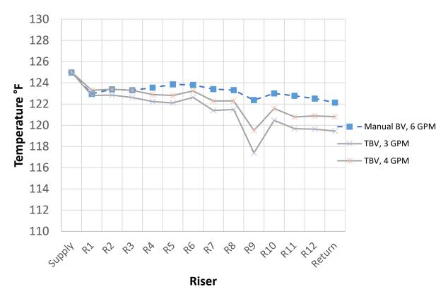
Figure 62: Balancing valve performance at select conditions.
