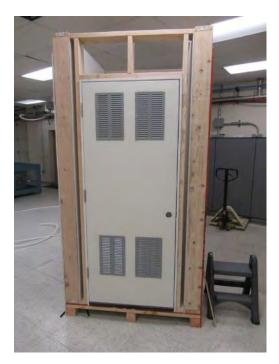
Figure 46: Ventilation grilles on the door of the closet used in laboratory tests.
