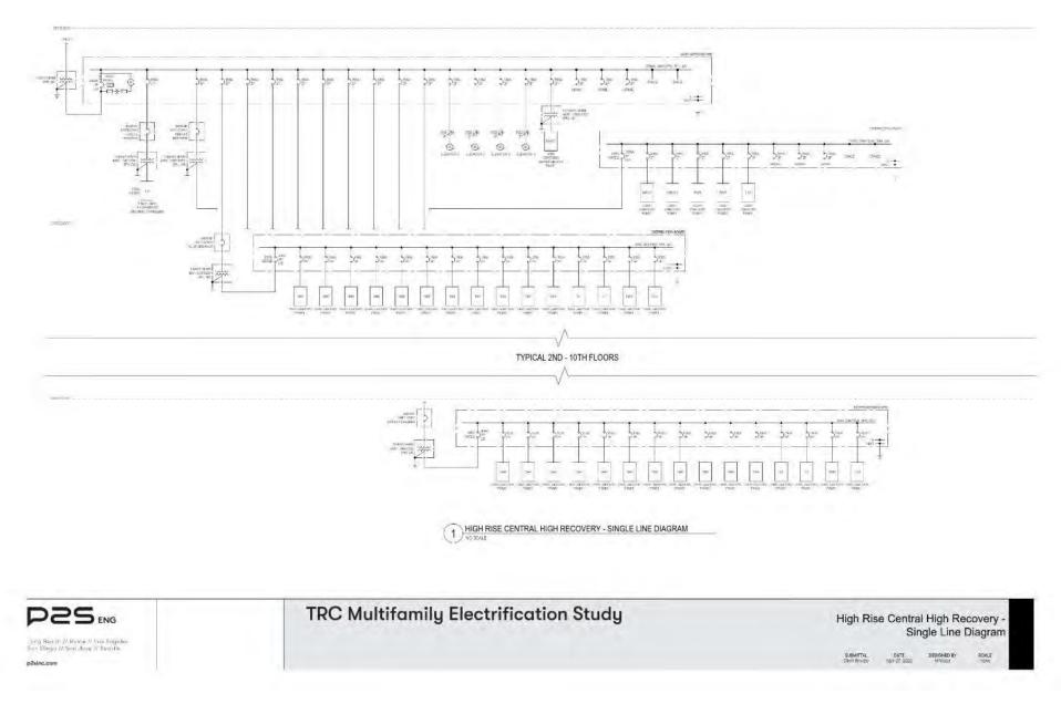
Figure 58: High-rise mixed use central high-recovery HPWH electrical SLD.
