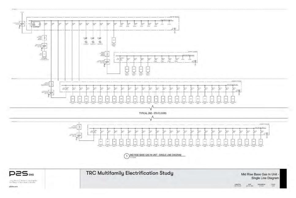
Figure 55: Mid-rise mixed use base case electrical SLD.
