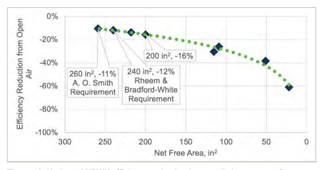
Figure 40: Unducted HPWH efficiency reduction in a small closet vs. net free area of vents connecting the DHW closet to larger interior spaces.
