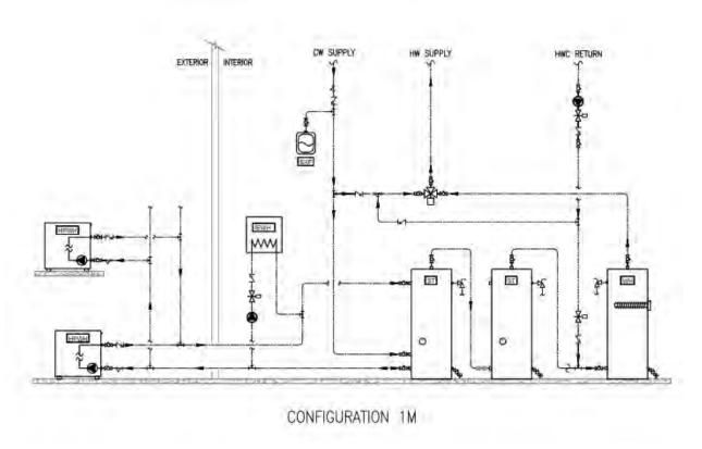
Figure 35: Single-pass primary with electric resistance water heater for temperature maintenance system.
