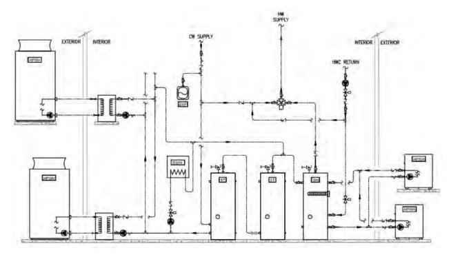
Figure 37: Single-pass primary with multi-pass in parallel for temperature maintenance system design.
