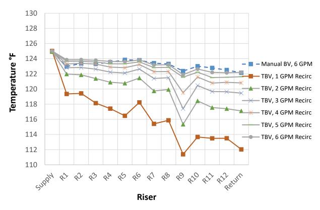
Figure 61: Balancing valve performance at multiple conditions.
