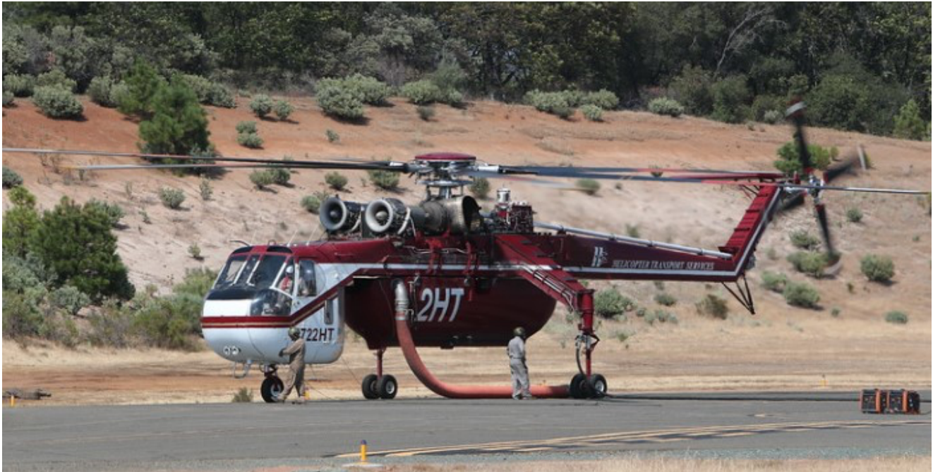
FIGURE 11: TYPE 1 HELITANKER WITH 2,400-GALLON TANK
