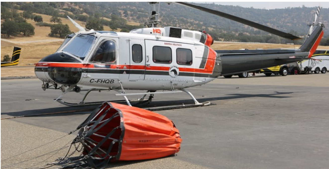
FIGURE 12: TYPE 2 WITH 360-GALLON BUCKET
