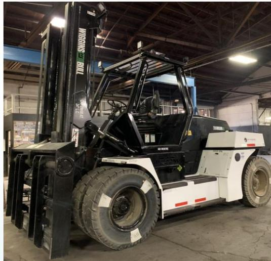
Source: Wiggins, battery electric forklift
