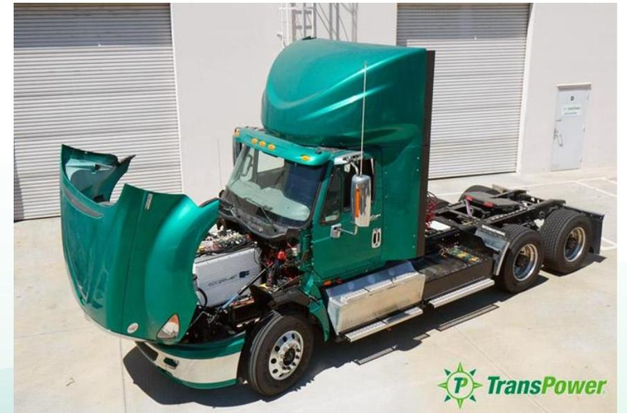
TransPower Battery ElecTruck™ Drayage Truck (EDD-2)
