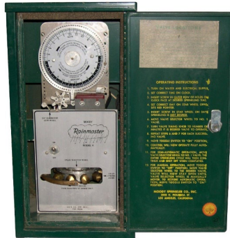
Figure 2-1: 1950s Landscape Irrigation Controller
