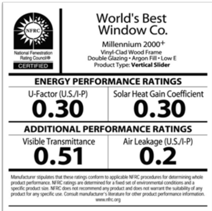
Figure 3: Window label for energy performance rating and proof of NFRC certification
