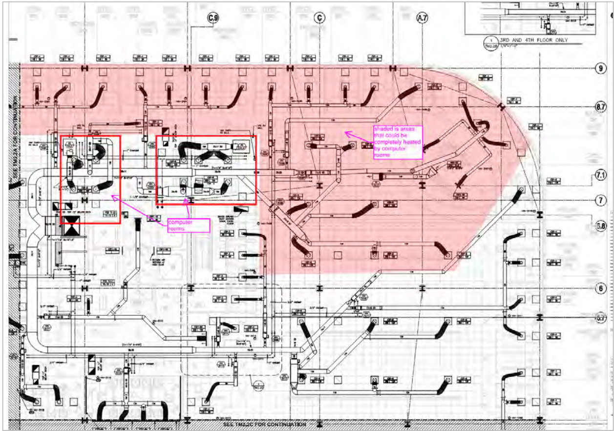
Figure 44: Typical Office Computer Room showing Heat Recovery Opportunity, Example 1
