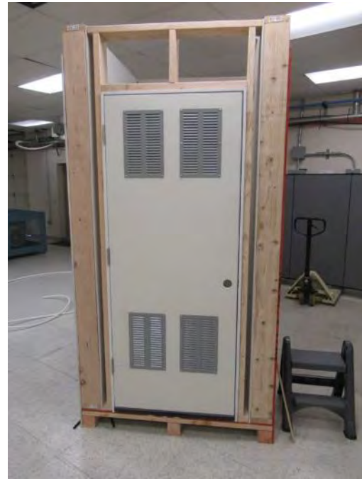
Figure 23: Ventilation grilles on the door of the closet used in laboratory tests.
