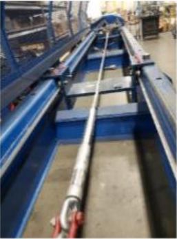
Figure 1 – Tensile load test setup for complete conductor.
