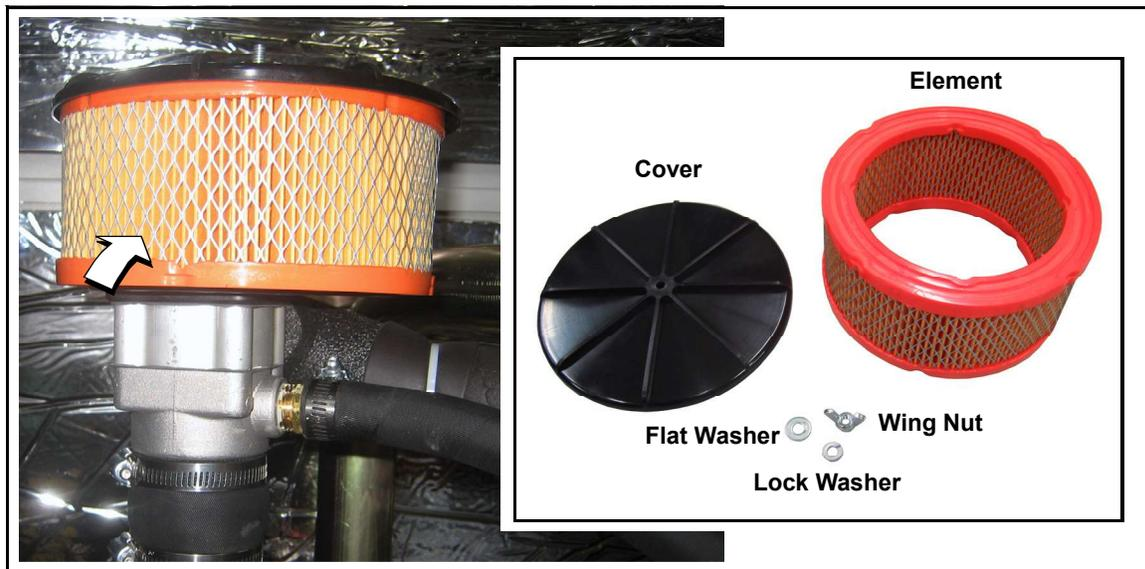
**Figure 5-13. Air Cleaner Cover and Filter Element**
