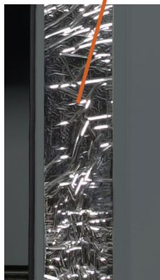
**Dense, Closed-Cell Foam Insulation with Reflective Silver Mylar Layer**
