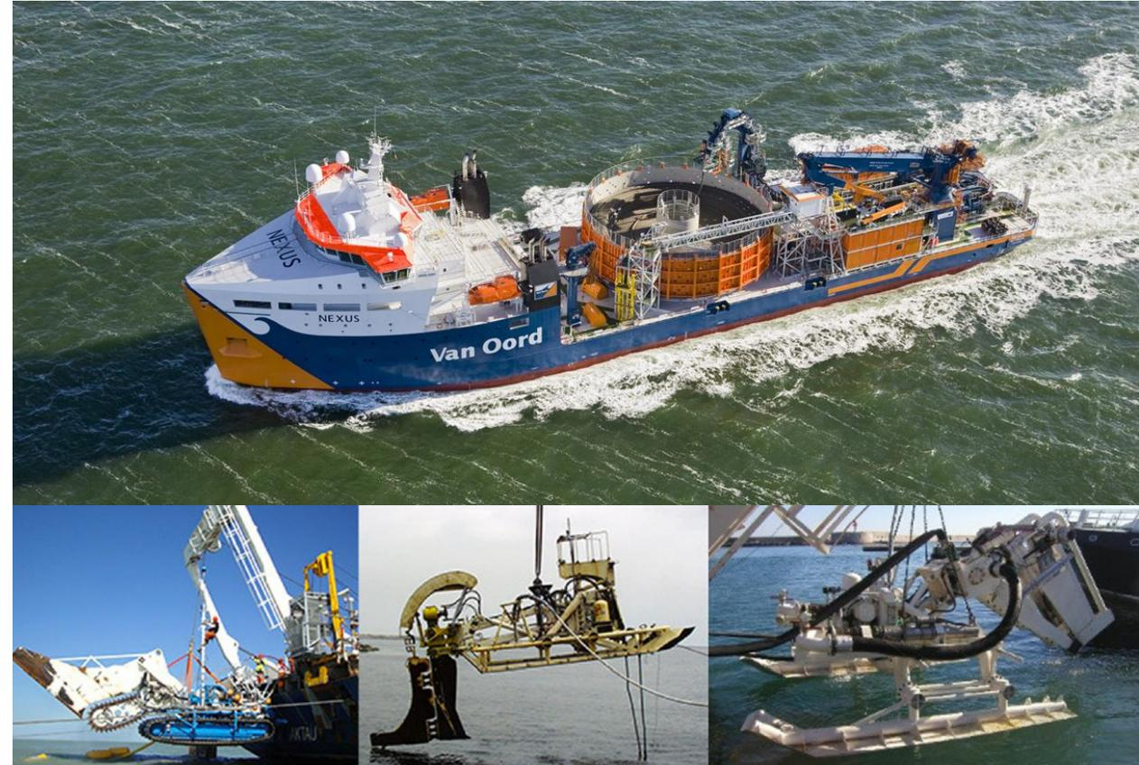
Fig. 1. Wheel cutter (left); Plough (centre) and Towed Jetting Vehicle (right) (courtesy: [www.ldravocean.com](http://www.ldravocean.com)).
