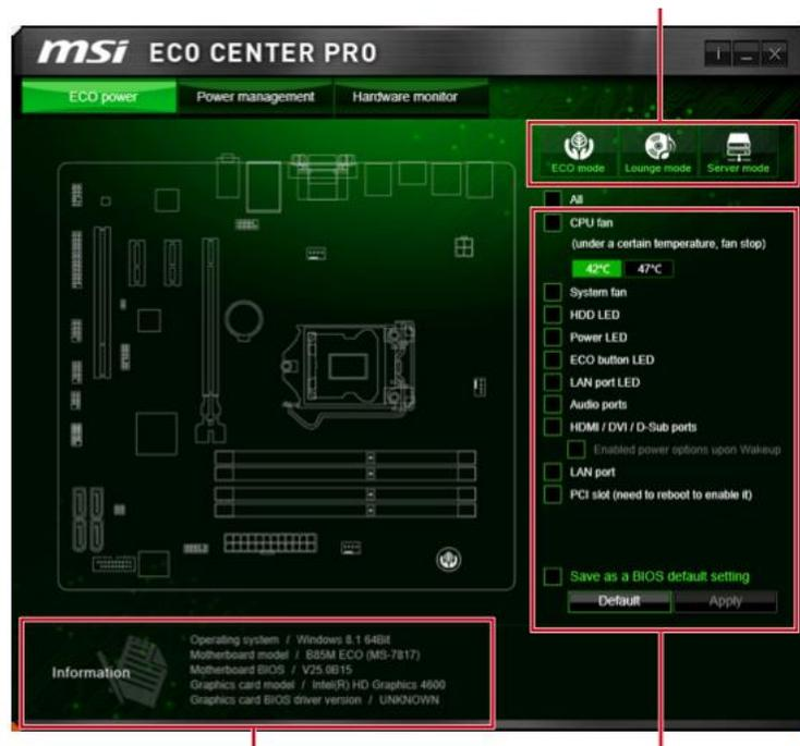
Figure 3 ECO power screen of ECO Center Pro
