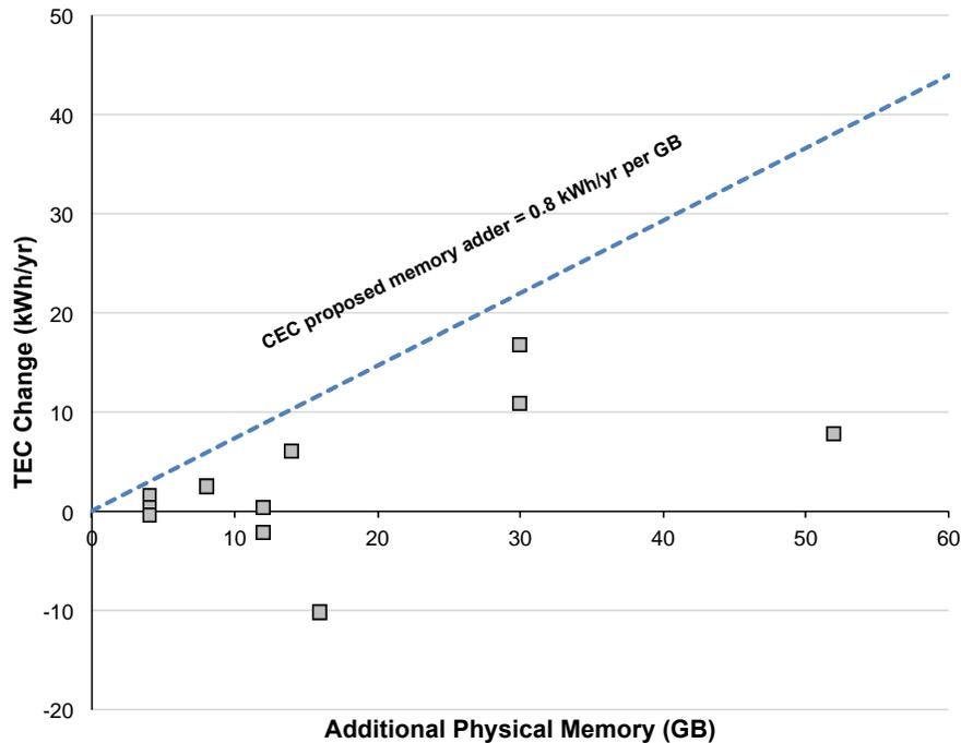
**Figure 3.10: Incremental TEC consumed by desktop computers with additional installed memory. Source: ENERGY STAR qualifying products list, 2015**
