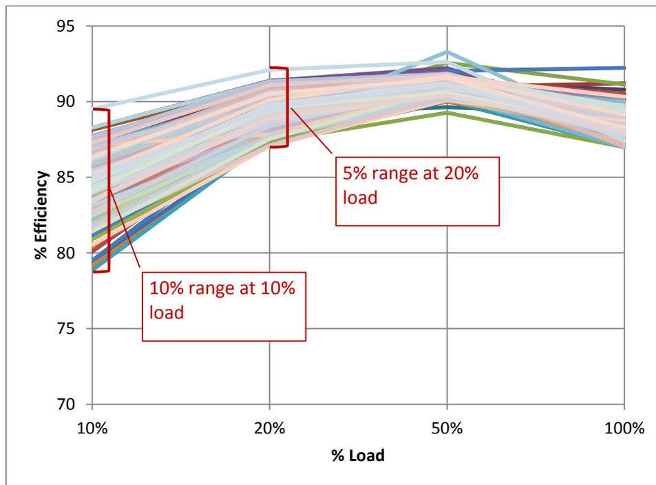
Figure 5.1: Efficiency Profiles of 80-PLUS GOLD Power Supplies
