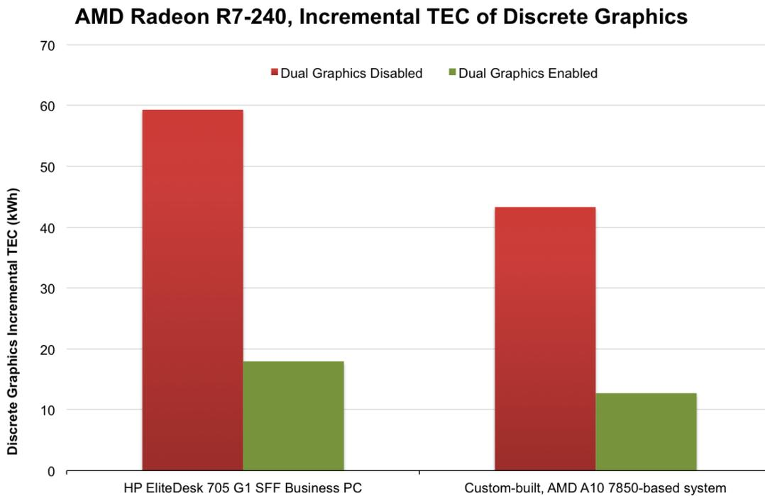
**Figure 3.8: Measurements of Radeon Dual Graphics incremental TEC impacts compared to baseline systems without discrete graphics**
