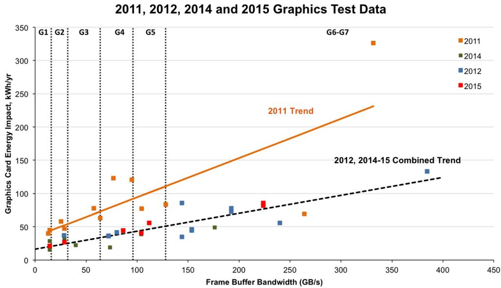
Figure 3.7: IOU, NRDC and CLASP measurements of dGfx, 2011 - 2015
