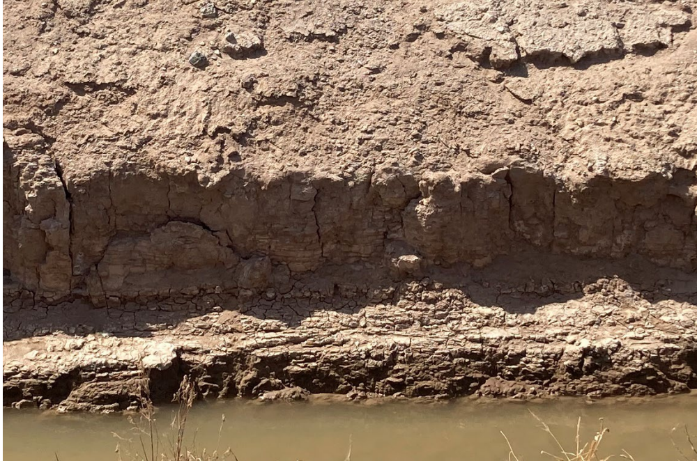
Photograph 3: Interbedded mudstone and siltstone of Lake Cahuilla bed sediments exposed at the bottom of the canal on the north side of Schrimpf Road. Facing south.
