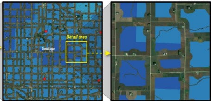
Detailed view of exclusion analysis; areas around roads, structures and streams
