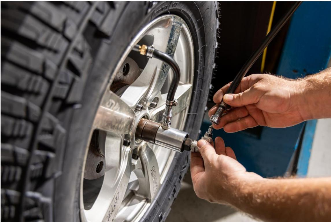
Photograph A5.2: Connecting Tire to Air Pressure
