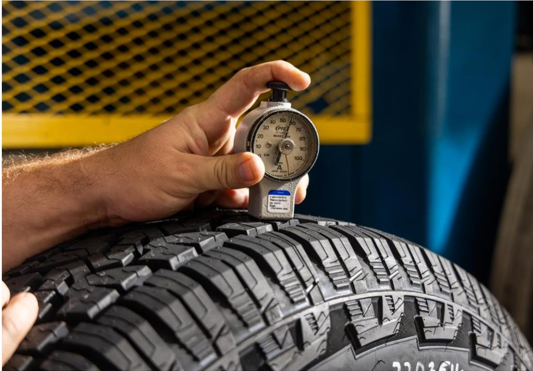
Photograph A5.3: Measuring Tread Hardness
