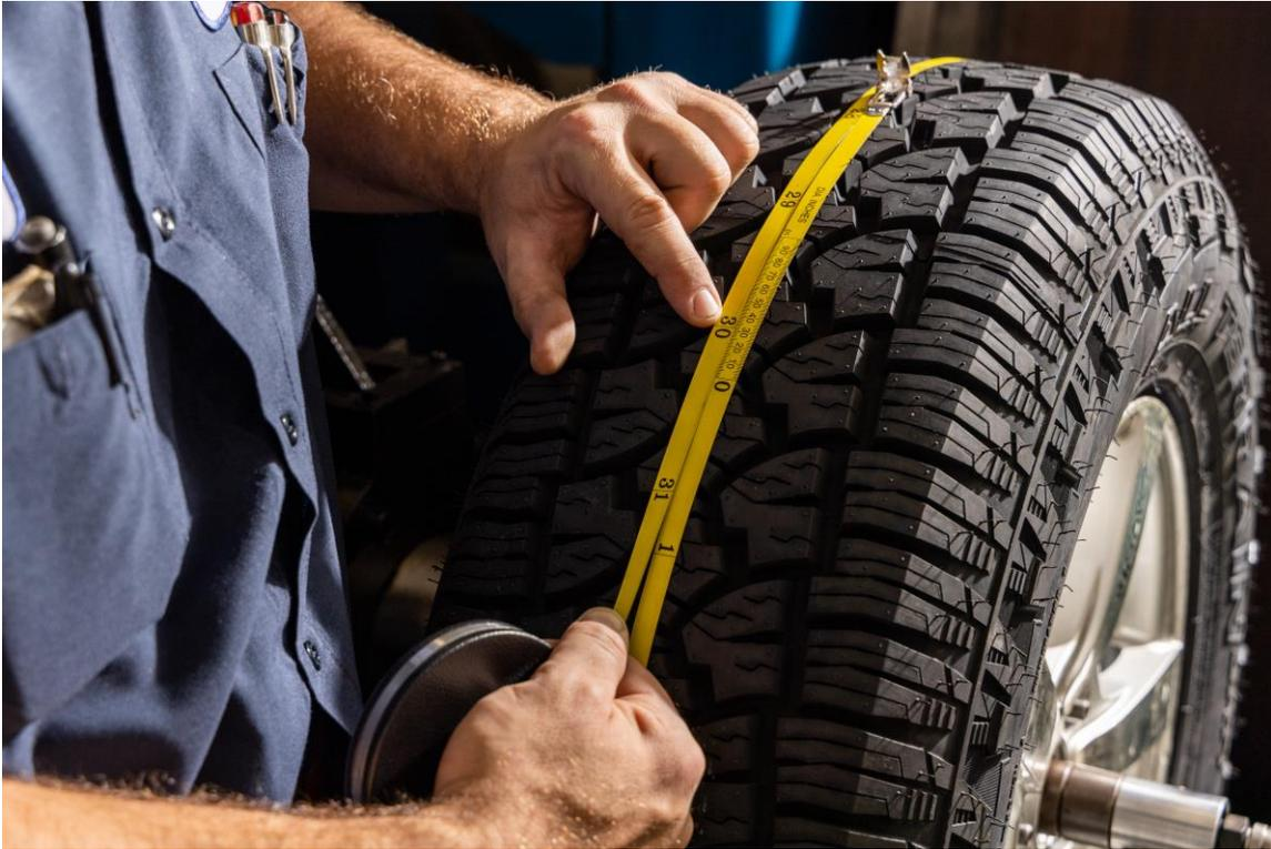
Photograph A5.5: Measuring Outside Diameter
