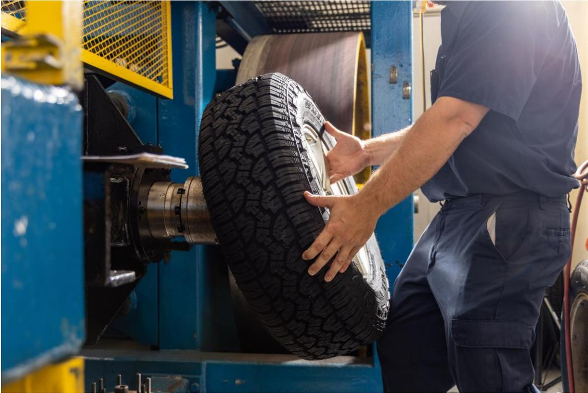
Photograph A5.1: Mounting Rolling Resistance Tire
