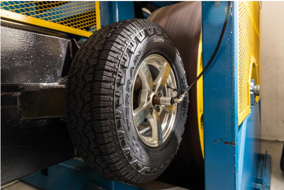
Photograph A5.6: Tire Ready for Testing
