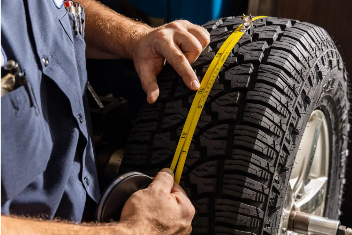
Photograph A5.5: Measuring Outside Diameter
