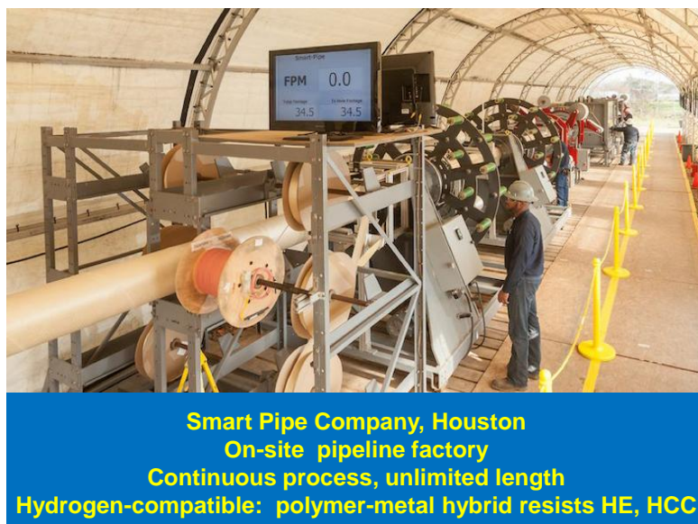
Figure 15. See Figs. 13, 14, 31-37. Onsite continuous-process factory produces custom composite pipeline in unlimited length, for pull-through rehabilitation or re-purposing of extant pipelines for high-purity, high-pressure, variable-pressure, GH 2 service including VER-source, or for new-builds. A non-ferrous metal foil, Cu or Al, may be built into pipe wall as the GH 2 permeation barrier; foil seams perhaps laser-welded. FRP reinforced overwrap: MAOP hoop strength.
