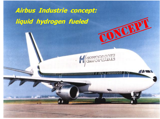
Figure 24. Aviation may require LH2 fueling, probably via short pipelines from local bulk storage. GH2-fueled smaller aircraft, up to ~ 70 pax class prop-driven, will pioneer. Hundreds of airports must provide, or ad hoc access, H2 fuel for accidental and emergency diversions from destination airports. A continental GH2 pipeline network will be required for aviation maturity on H2 fuels: GH2 and LH2. [44, 46, 48, 50]
