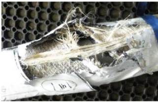
Burst Test Failure
