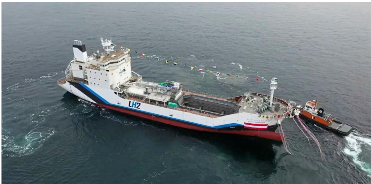
Figure 41. Bunkering liquid hydrogen (LH2) fuel to cruise ships and other large marine vessels will require short-distance LH2 pipelines from the liquefier plants to the bunkering tanker docks. Bottom photo is the world's only oceangoing LH2 tanker, by Kawasaki Heavy Industry. [79]
