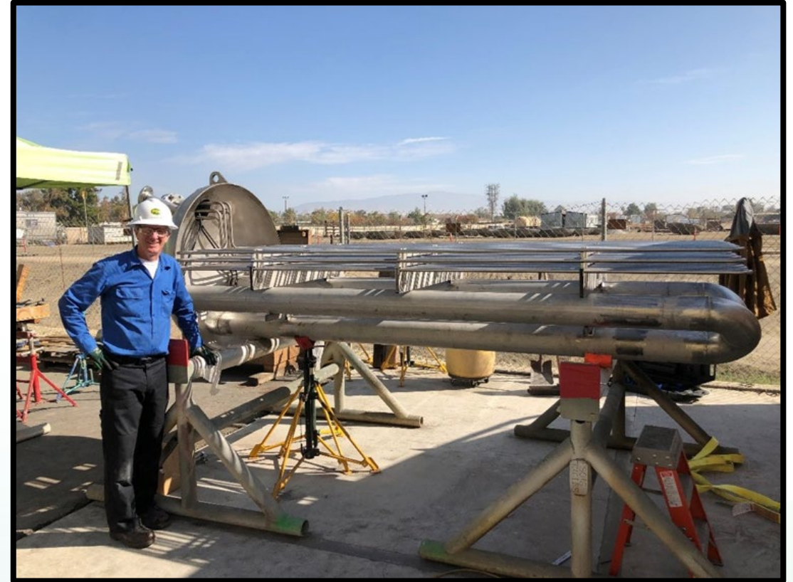
Element 16 successfully commissioned the CCHP-TES system at its own commercial facility in Arcadia, CA. (Source: Element 16 Technologies, Inc.)
