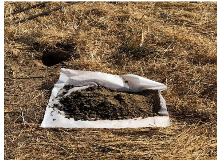
Photo 16: (SP-8) Soil cuttings from hand augering to 2 feet bgs
