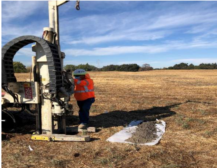
Photo 13: (SP-5) Direct push drilling to 20 feet bgs.
