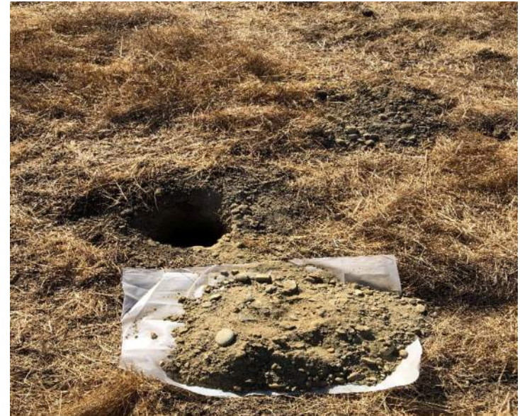
Photo 14: (SP-6) Soil cuttings from hand augering to 2 feet bgs.
