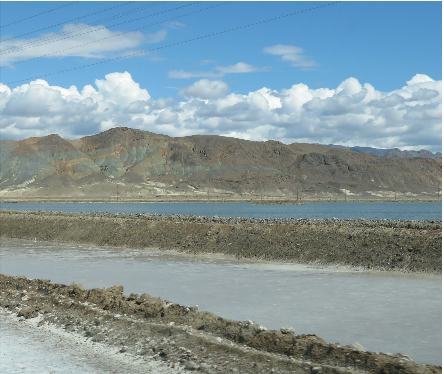
Evaporating Ponds, Silver Peak Lithium Mine. Photo © Ken Lund, cropped version used under an Attribution-ShareAlike 2.0 Generic Creative Commons (CC BY-SA 2.0) license.
