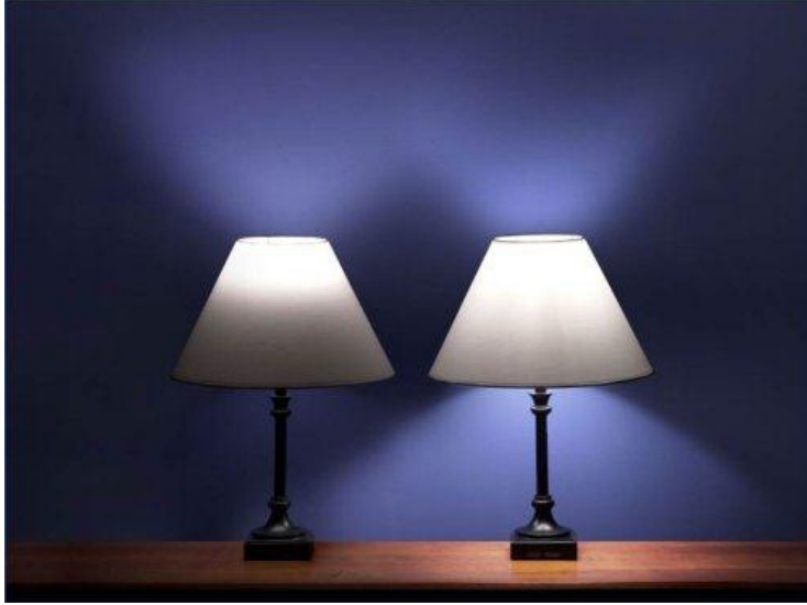
Figure 23 Light distribution comparison of two LED A-lamps in table lamps
