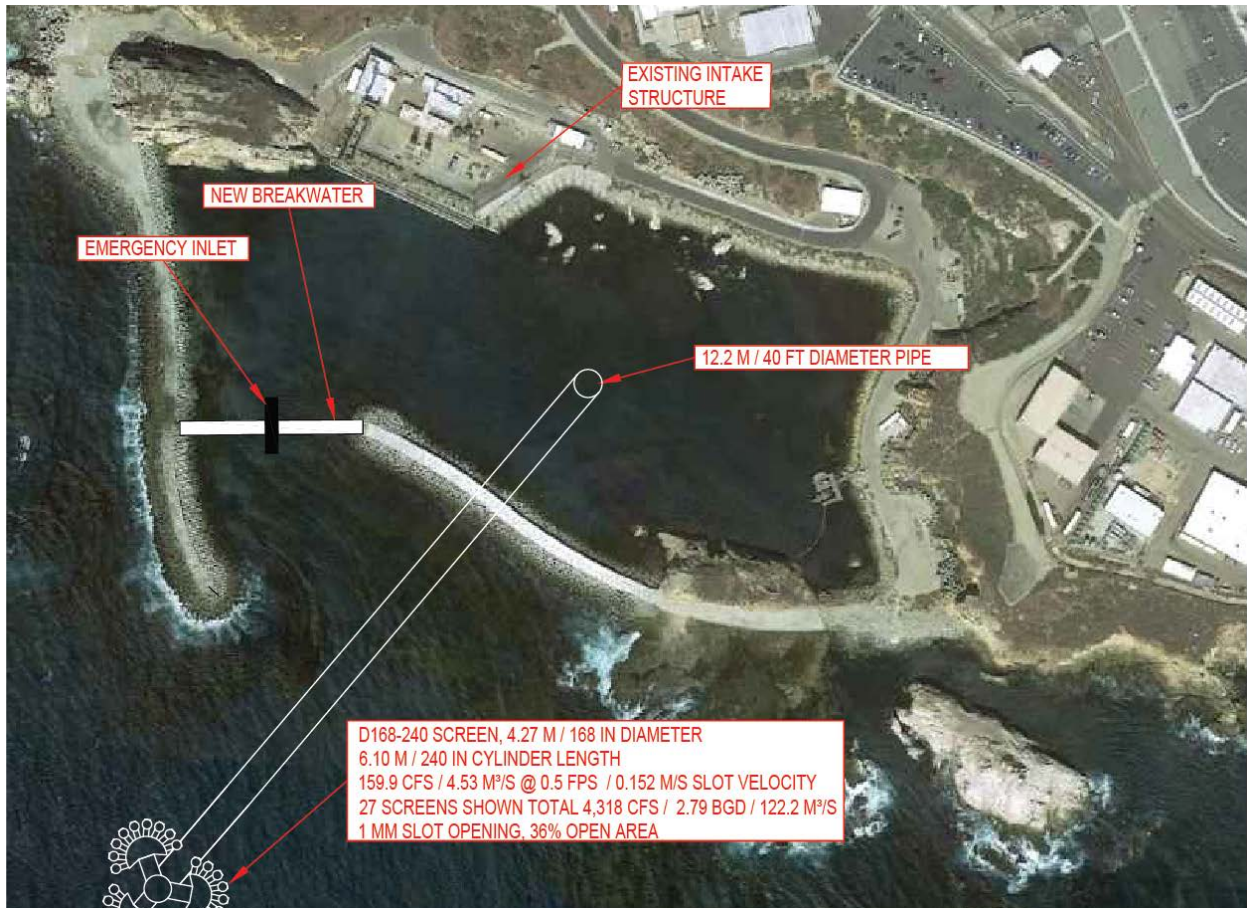
Figure 2-15: Aerial view of the plant with extended breakwater to isolate lagoon, emergency inlet structure, tunnel extending offshore, and wedgewire screen array for Option 1 (Intake Screens, Inc. Report)
