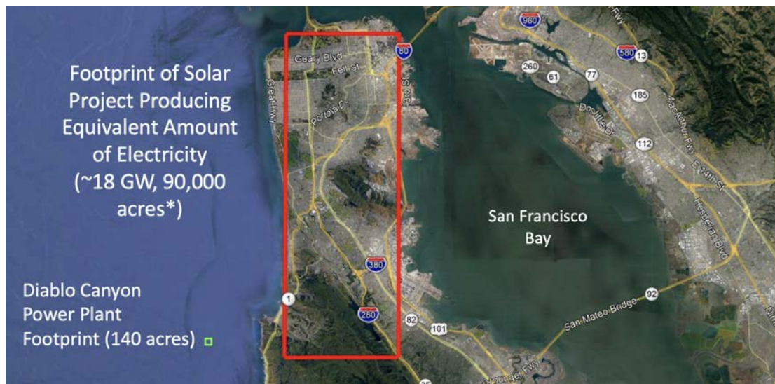
Figure 1-7: Hypothetical spatial footprint of 18 GW of PV compared to the San Francisco metro area (Credit: Lucid Catalyst LLC)
