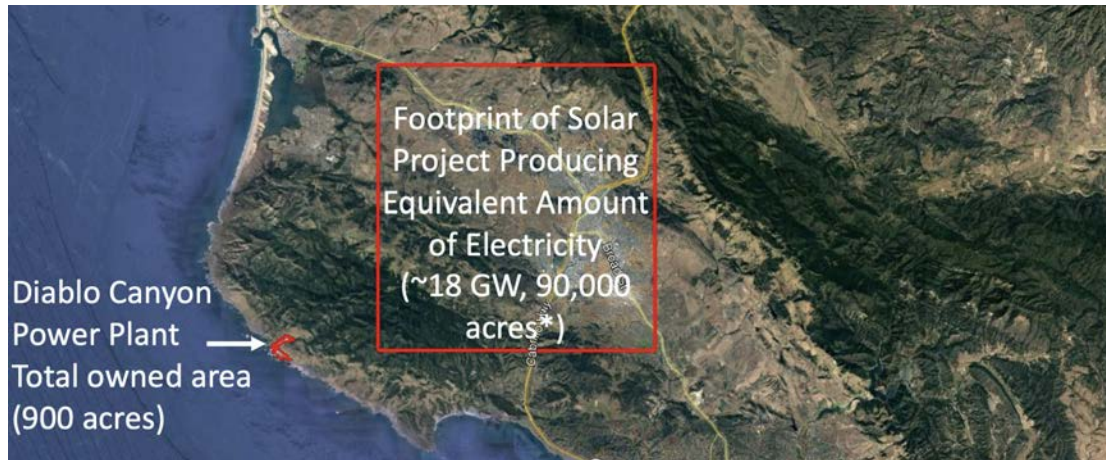
Figure 1-6: Hypothetical spatial footprint of 18 GW of PV near the Diablo Canyon plant (Credit: Lucid Catalyst LLC)
