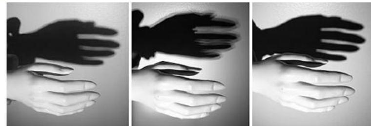
Figure 1-3 Shadows from (left) a large source (Halogen MR16), (center) multiple point sources (first generation LED MR 16 with 4 LEDs) and (right) single point source (GaN on GaN LED MR16) source
