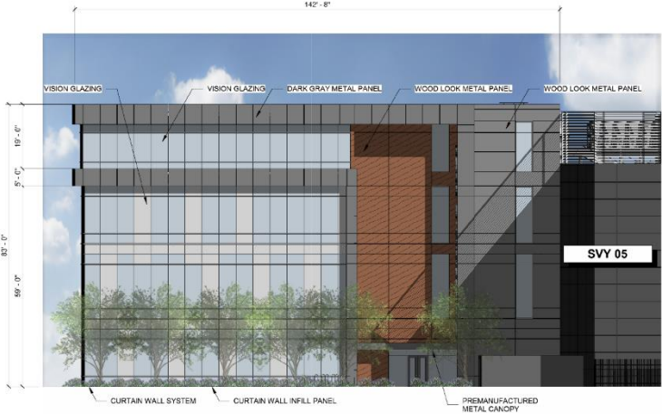
2 SVYAM - WEST ELEVATION - VIEW FROM RINGWOOD 1/16" = 1'-0"
