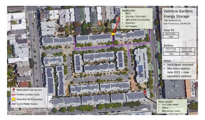
As shown in the following future microgrid schematic, the 1-BESS project is similar to the 2-BESS project but does not require a recloser or a vault. Like the 2-BESS project, the 1-BESS project sets the stage for a potential Community Microgrid at the VGA complex — which can be created by adding a grid isolation switch that can be activated in the event of a grid outage, and using the solar+storage to maintain electrical power for the office and other critical loads.
