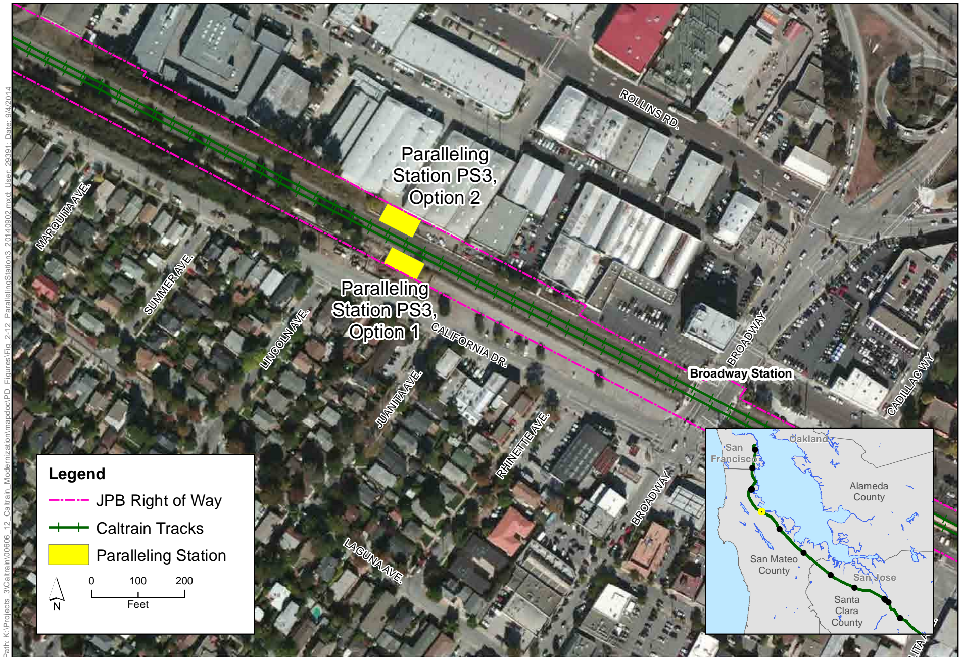
Figure 2-12 Proposed Paralleling Station 3 (PS3), Options 1 and 2, Burlingame Peninsula Corridor Electrification Project
