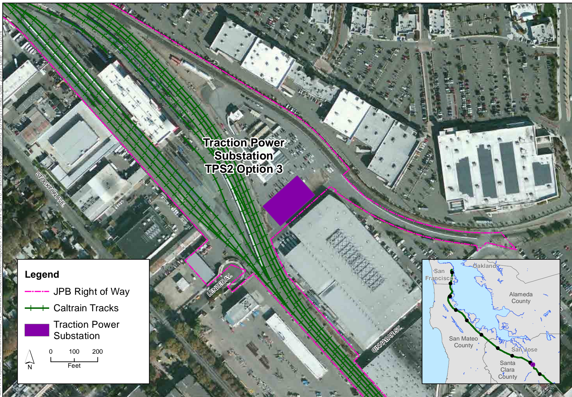
Figure 2-17b Traction Power Substation 2, Option 3 (TPS2, Option 3), San Jose Peninsula Corridor Electrification Project
