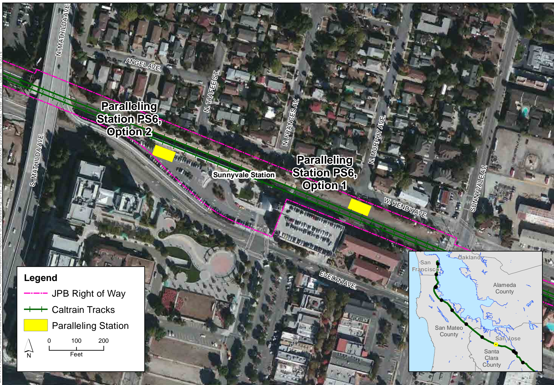
Figure 2-16 Proposed Paralleling Station 6, Option 1 & 2 (PS6, Option 1 & 2), Sunnyvale Peninsula Corridor Electrification Project
