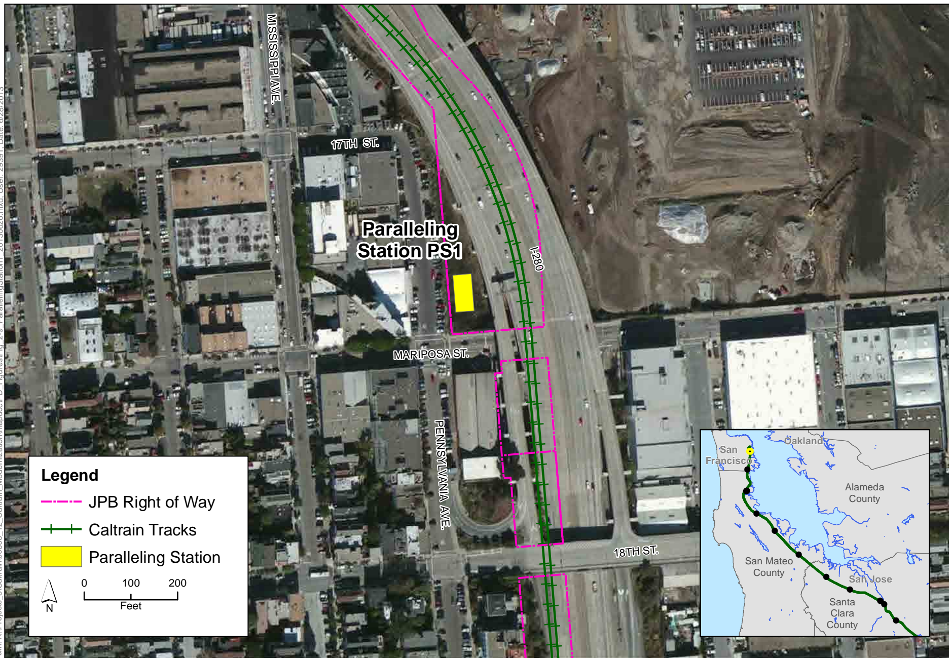
Figure 2-9 Proposed Paralleling Station 1 (PS1), San Francisco Peninsula Corridor Electrification Project
