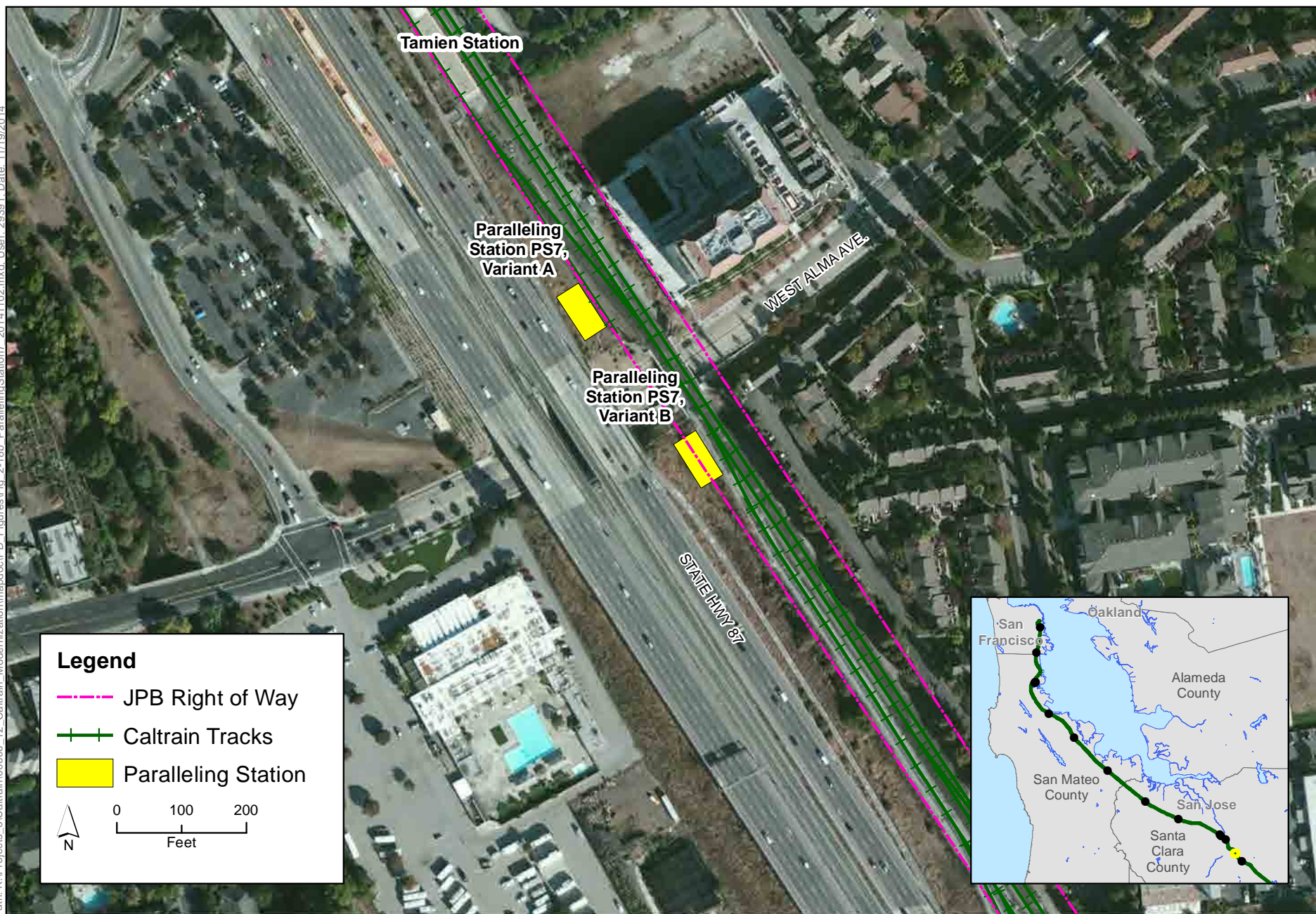
Figure 2-18b Proposed Paralleling Station 7, Variants (PS 7, Variants), San Jose Peninsula Corridor Electrification Project
