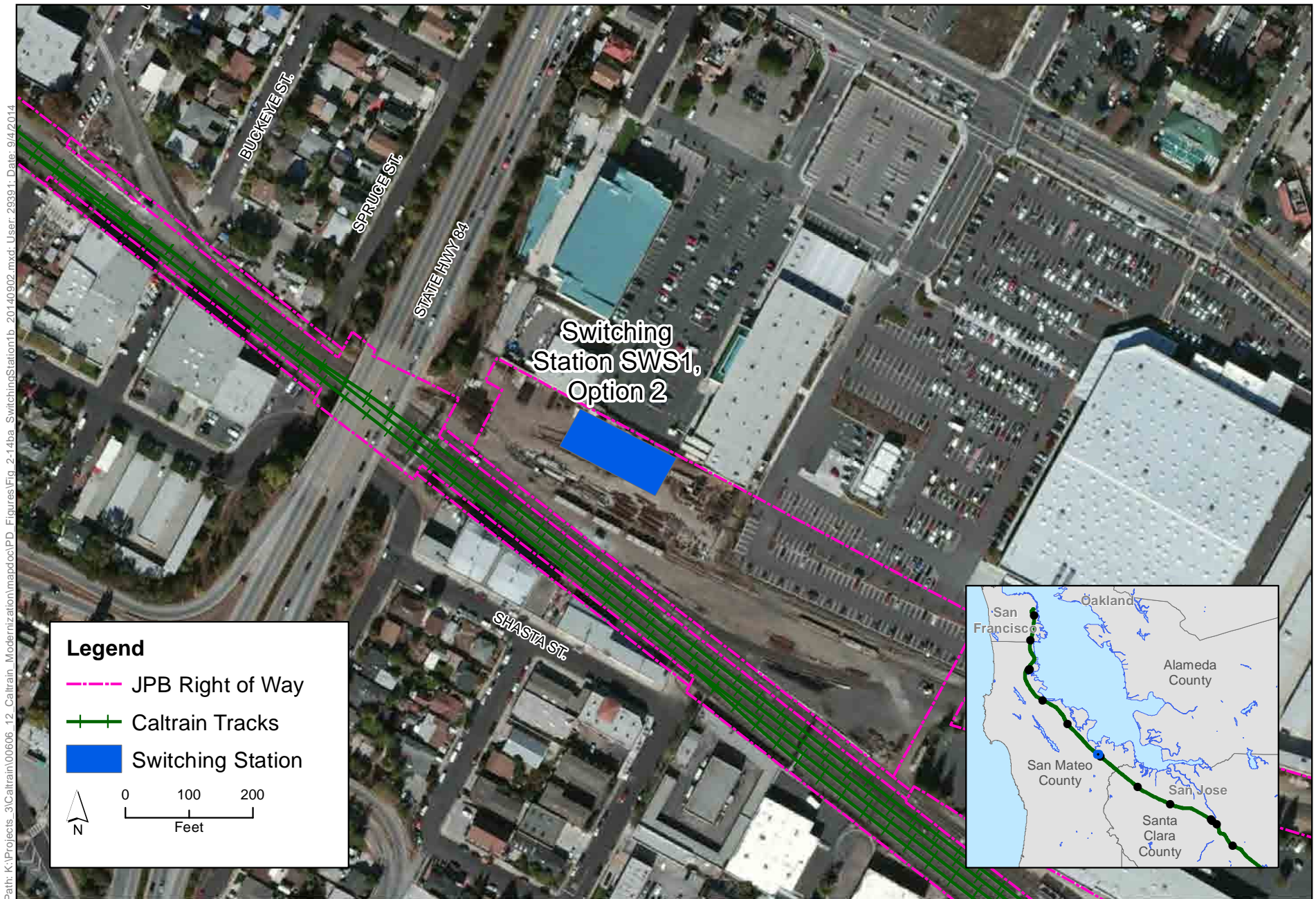
Figure 2-14b Proposed Switching Station 1, Option 2 (SWS1, Option 2), Redwood City Peninsula Corridor Electrification Project
