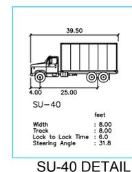
NOTE THAT SU-40 IS USED TO SIMULATE A GARBAGE TRUCK FOR THE PURPOSE OF THIS DRAWING.
