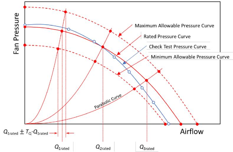
Figure 10.1 — Application of Airflow Tolerance
