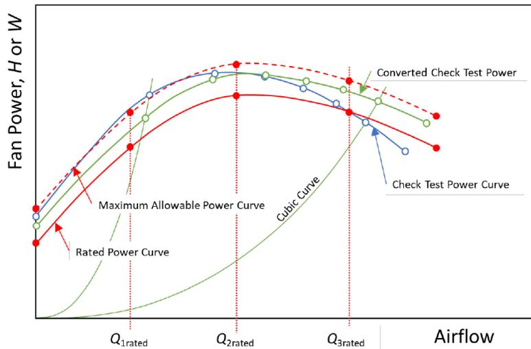
Figure 10.2 - Application of Power Tolerance
