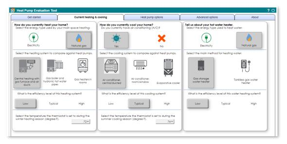
Users may specify their current space heating and cooling system and water heating for comparison with heat pump options.
