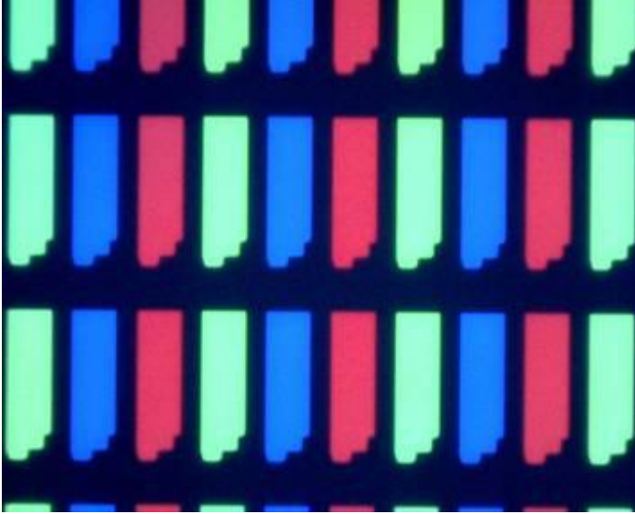
Figure 4.3 Micrograph of a twisted nematic LCD panel, an LCD type that is commonly used in computer monitors 2
