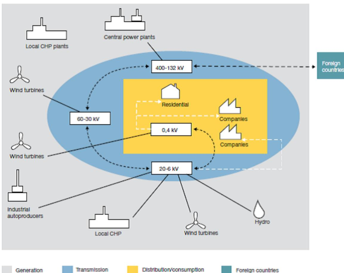
Figure 3: Structure of the grid in Denmark.
