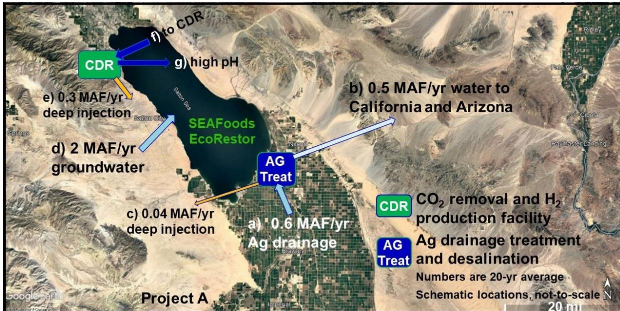
Fig. 1 – Filling and restoring the Salton Sea with local groundwater – Aerial schematic
