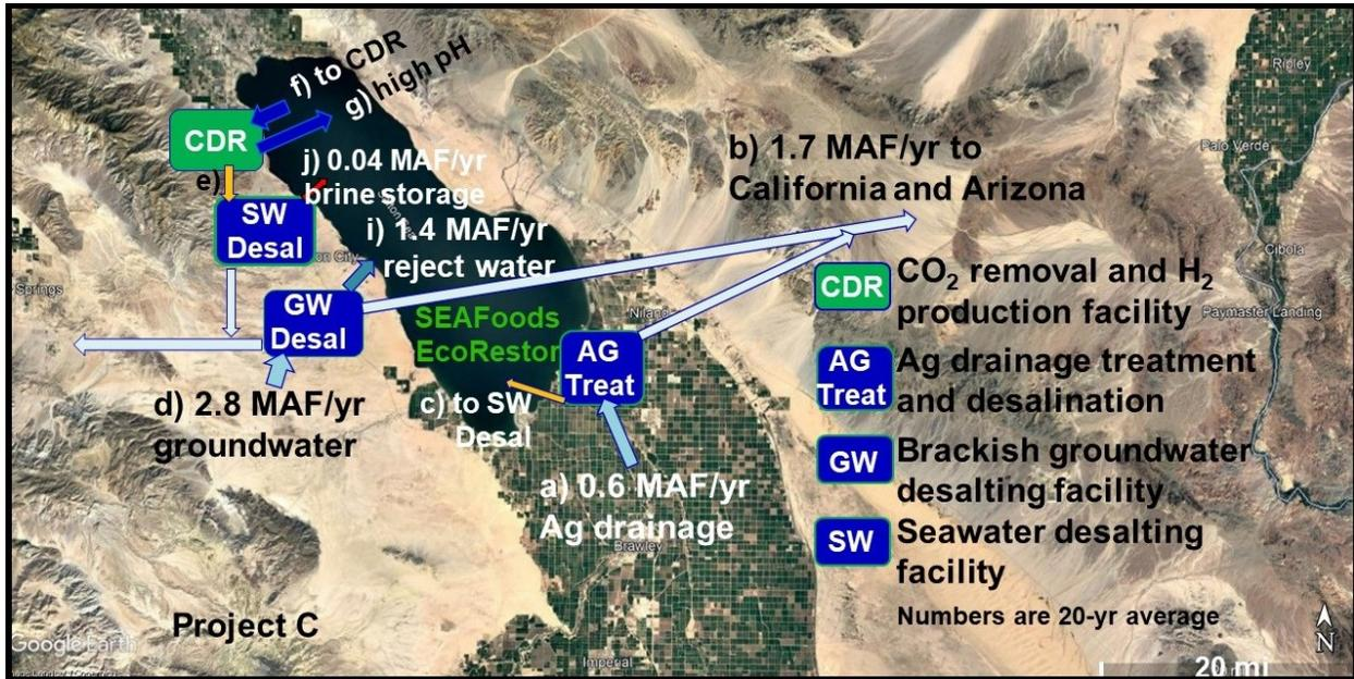
Fig.5 – Filling and restoring the Salton Sea with in-sea salt storage – Aerial schematic
