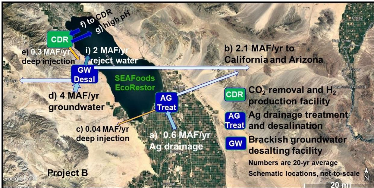
Fig. 3 – Filling and restoring the Salton Sea with improved water supply – Aerial schematic
