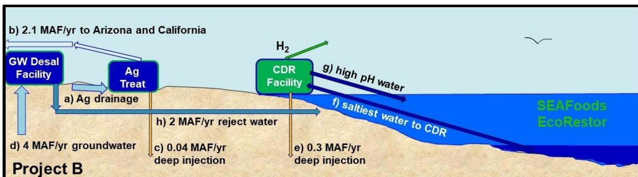
Fig. 4 – Filling and restoring the Salton Sea with improved water supply – Elevation schematic
