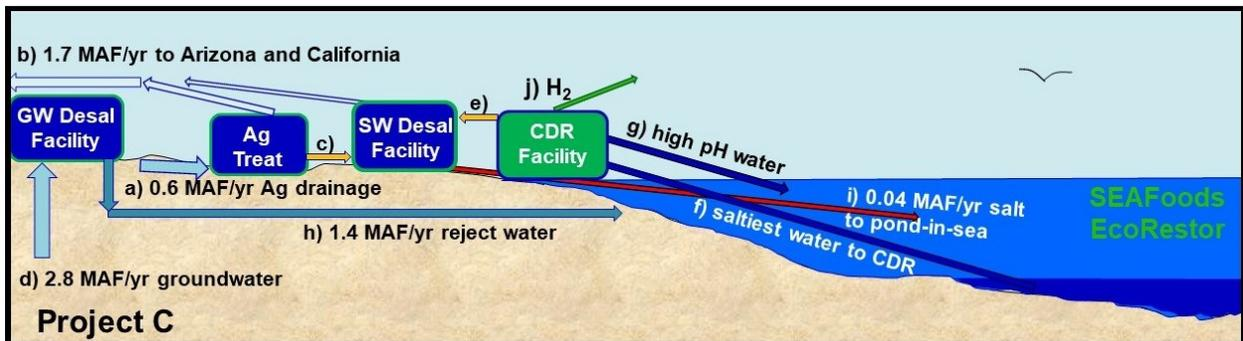
Fig. 6 – Filling and restoring the Salton Sea with in-sea salt storage – Elevation schematic
