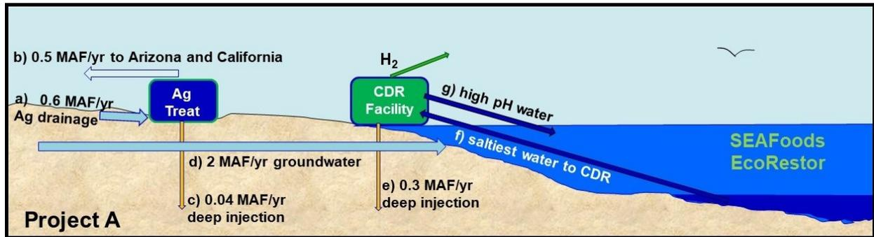
Fig. 2 – Filling and restoring the Salton Sea with local groundwater – Elevation schematic
