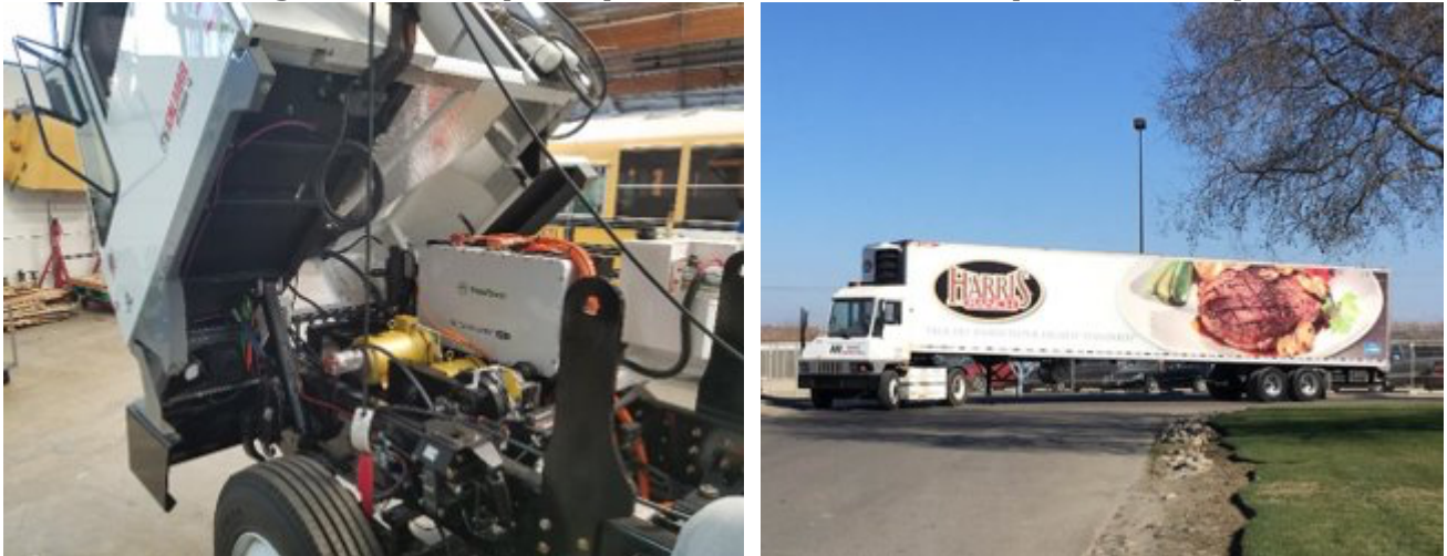
Figure 5: Heavy-Duty Electric Yard Tractor (TransPower)
