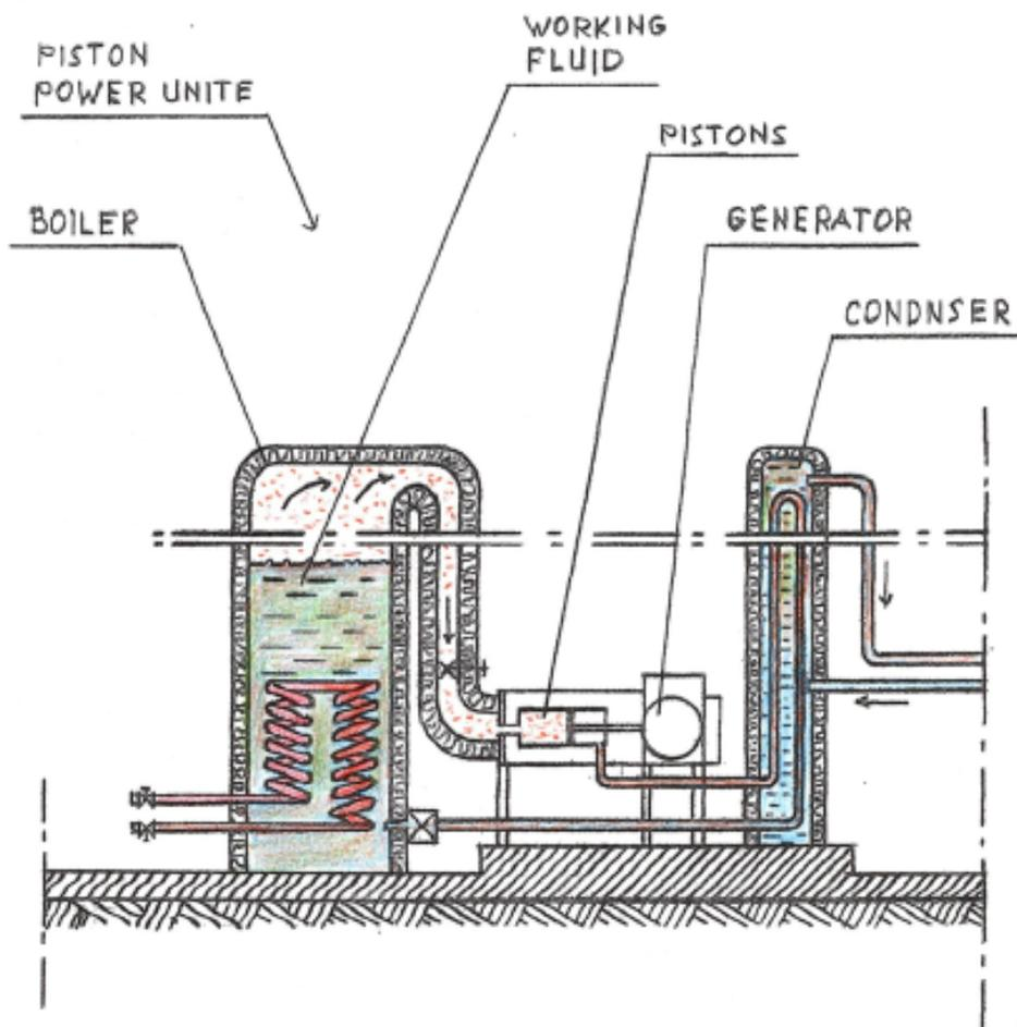
**FIG. 7** – Schematic Cross-sectional View of a Power Unit
