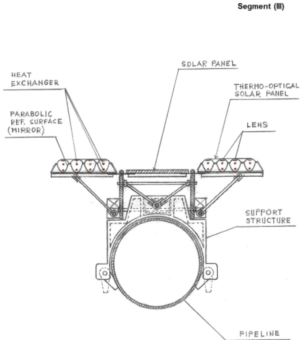
**FIG. 2 – Cross-sectional View of a Solar Panel Assembly**
