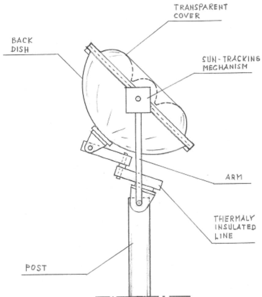
**FIG. 5** – Side View of a "Thermo-Optical Solar Dish"
