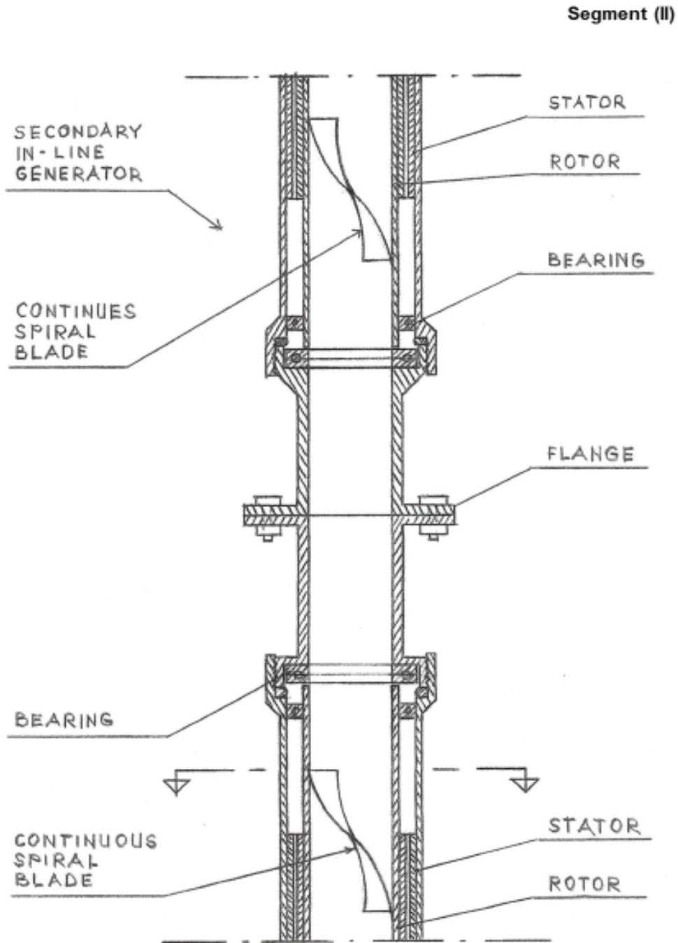
**FIG. 7 – Cross-sectional longitudinal View of the Secondary In-Line-Pump/ Generator**
