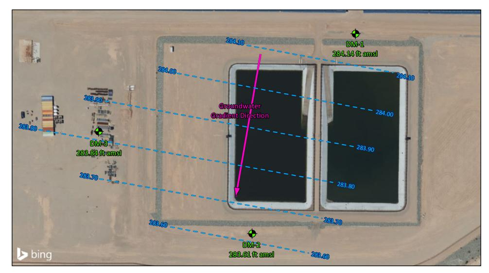
Groundwater Elevation Contour Lines
