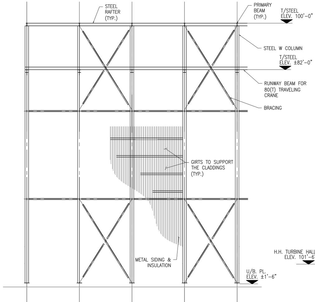
STRUCTURAL STEEL ELEVATION VIEW
