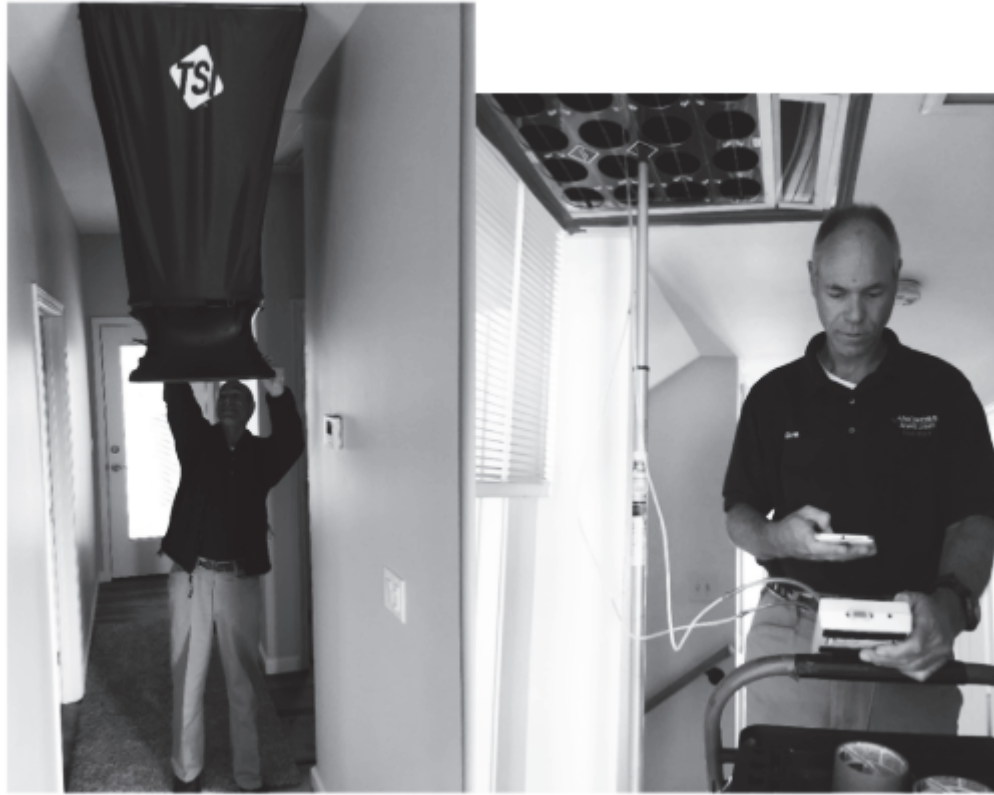
Figure 11-33: System Airflow Rate Measurement Using Flow Capture Hood (On Left) and Flow Grid (On Right) - Photo Courtesy of Bruce Cheney
