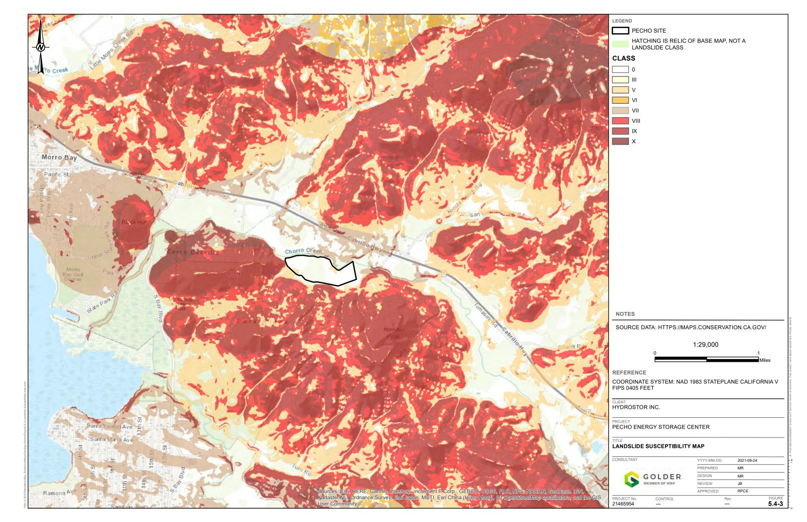
As noted, Figure 5.4-2 identifies multiple areas surrounding the PESC project site boundary with surficial landslide deposits These landslide deposits were identified on the mountain slope face to the south of site and are mapped outside of the PESC project boundary.
