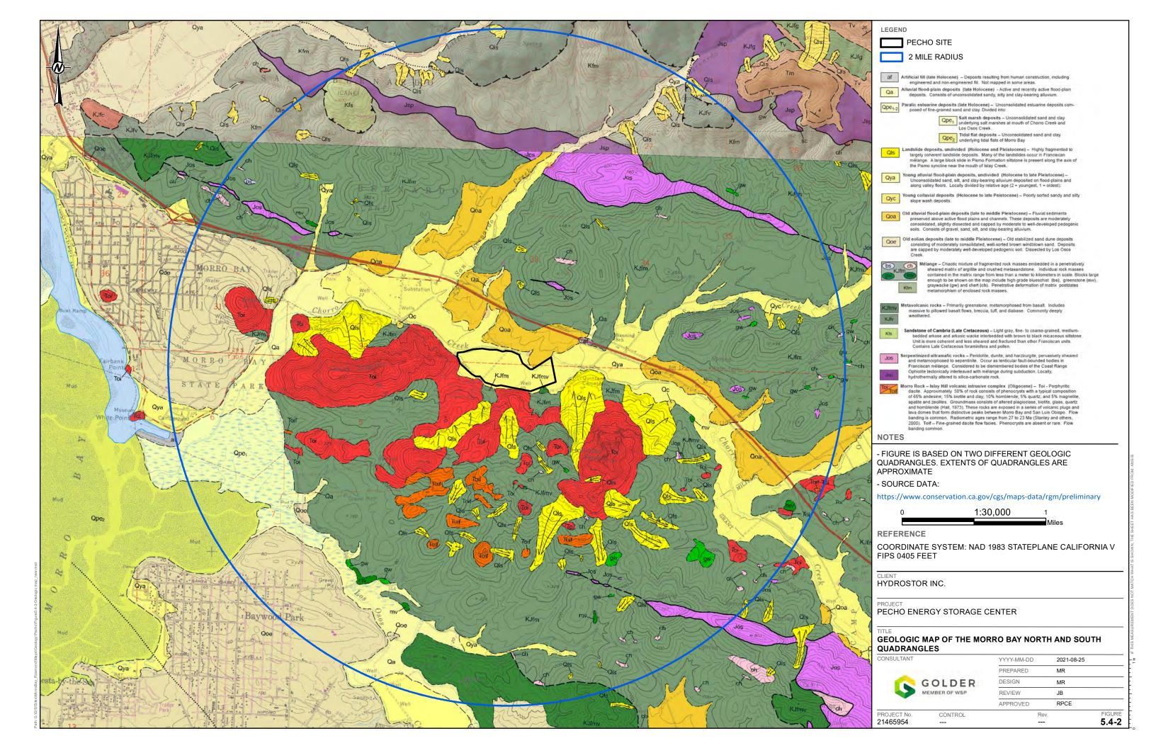
Site-specific hazard analyses (SHA) have not been performed for the site. However, a cursory assessment using the USGS Unified Hazard Tool (USGS 2014), assuming a 2475 return period and Site Class B (rock) conditions, indicates a peak ground acceleration (PGA) of 0.36g (where g represents acceleration due to gravity) and mean earthquake magnitude of 6.8.
