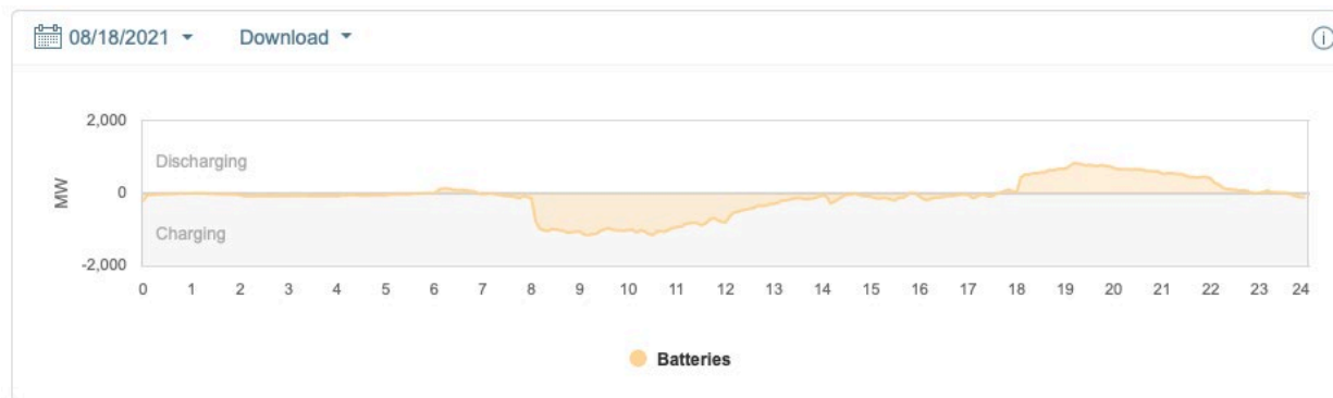
Fig. 2. 2 CAISO's use of batteries on August 18, 2021. 17
